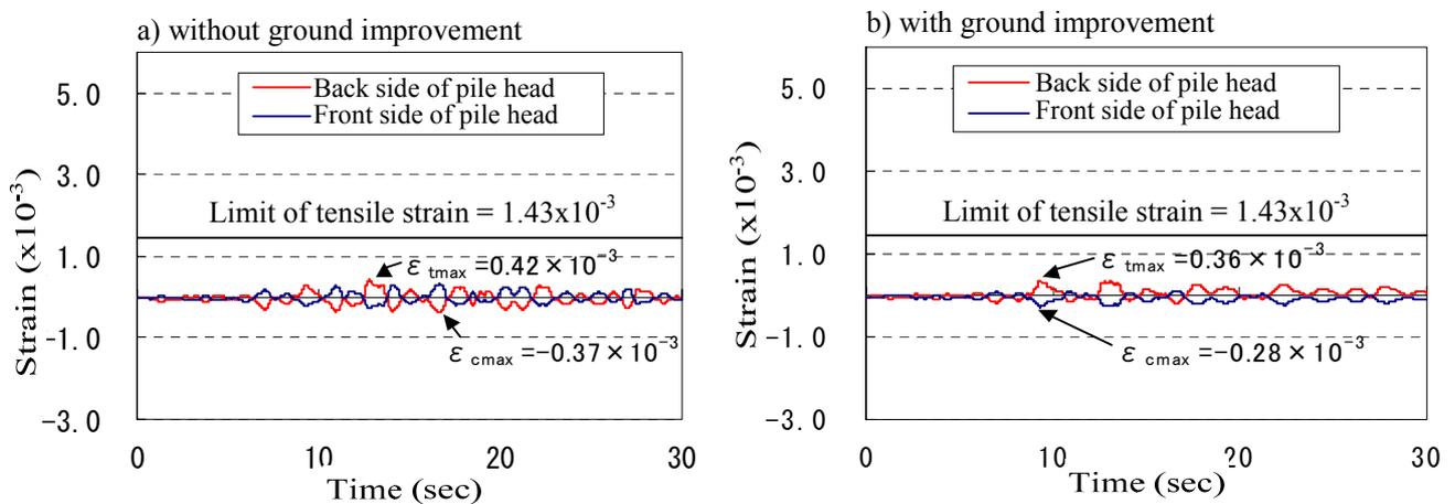
Figure 7 Time history of strain at pile head under Level 1 earthquake motion
