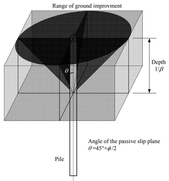
Figure 1 3-D image of the lateral resistance of pile foundation and the range of ground improvement
