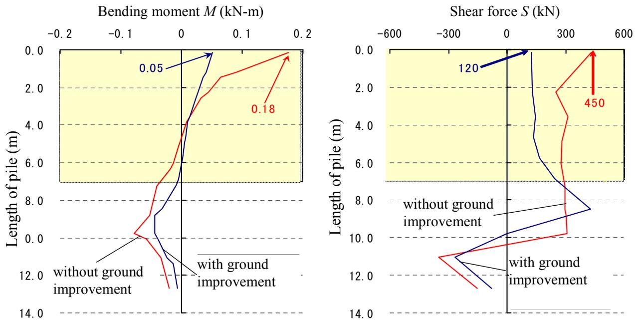
Figure 6 Distribution of sectional force of pile under Level 2 earthquake motion
