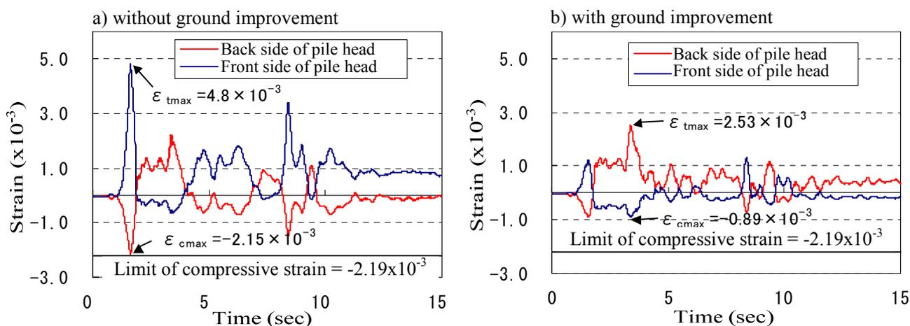
Figure 8 Time history of strain at pile head under Level 2 earthquake motion
