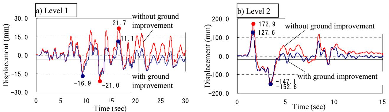
Figure 5 Time history of horizontal displacement of the footing
