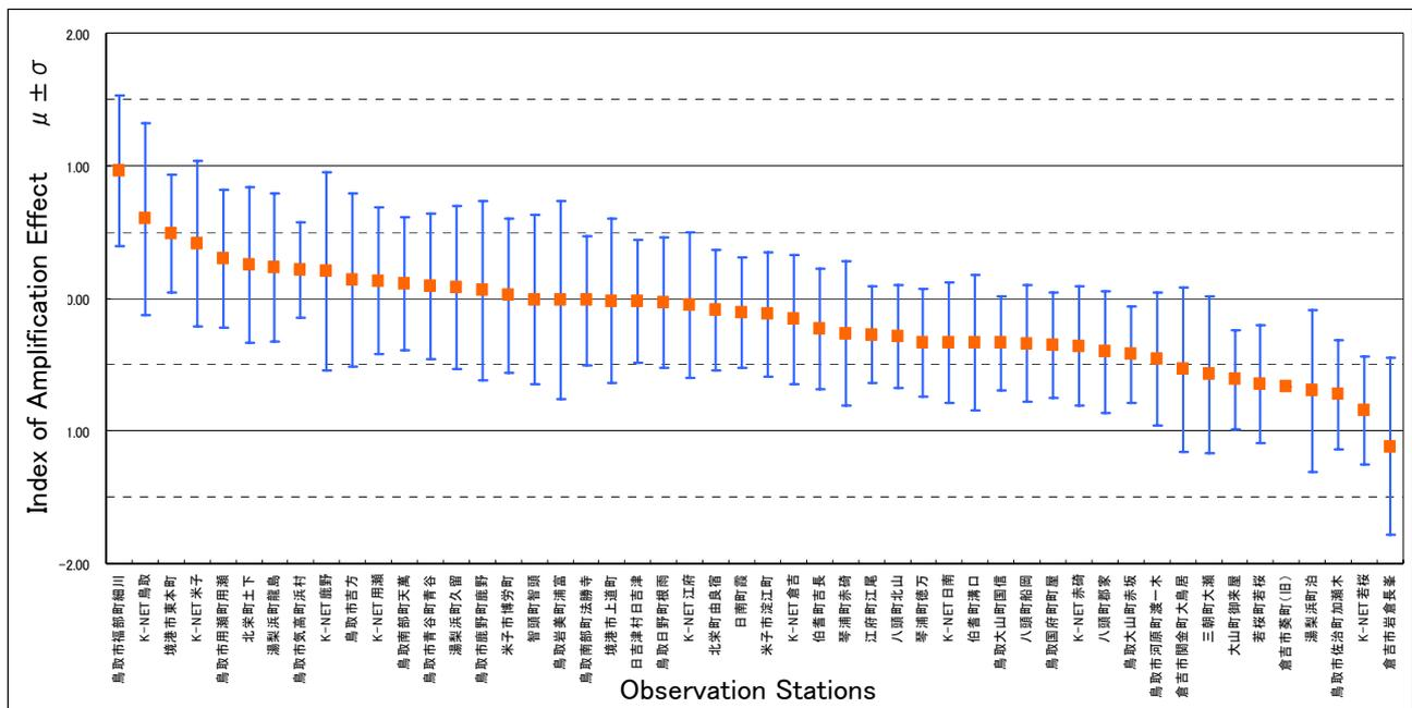
Figure 2 Mean of difference between estimated instrumental seismic intensity and observed value (the index of amplification effect) and the standard deviation of the estimate in the instrumental seismic intensity
