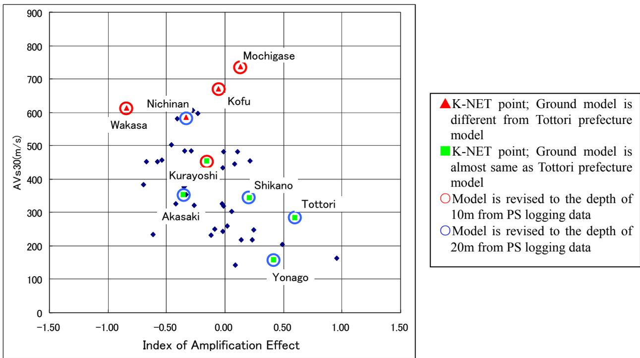
Figure 6 Comparison between the index of amplification effect and AVs30
