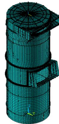
Fig. 3 Unit division of desulfurization tower
