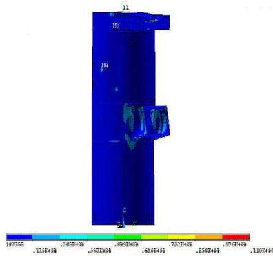
Fig.5 Stress pattern with seismic wave input in X direction
