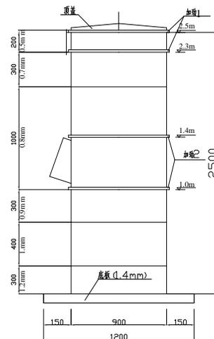
Fig. 2 Elevation drawing of desulfurization tower
