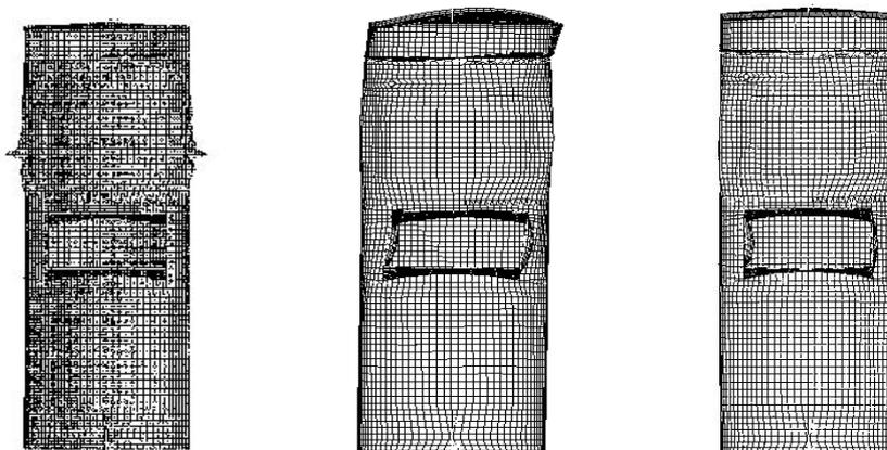
Fig. 4 Shaking modes of the first, the fourth and the ninth modal of desulfurization tower
