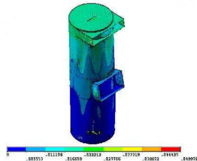
Fig.8 Structure deformation with seismic wave in Y direction
