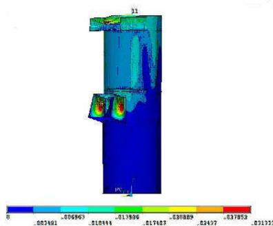
Fig.7 Structure deformation with seismic wave input in X direction
