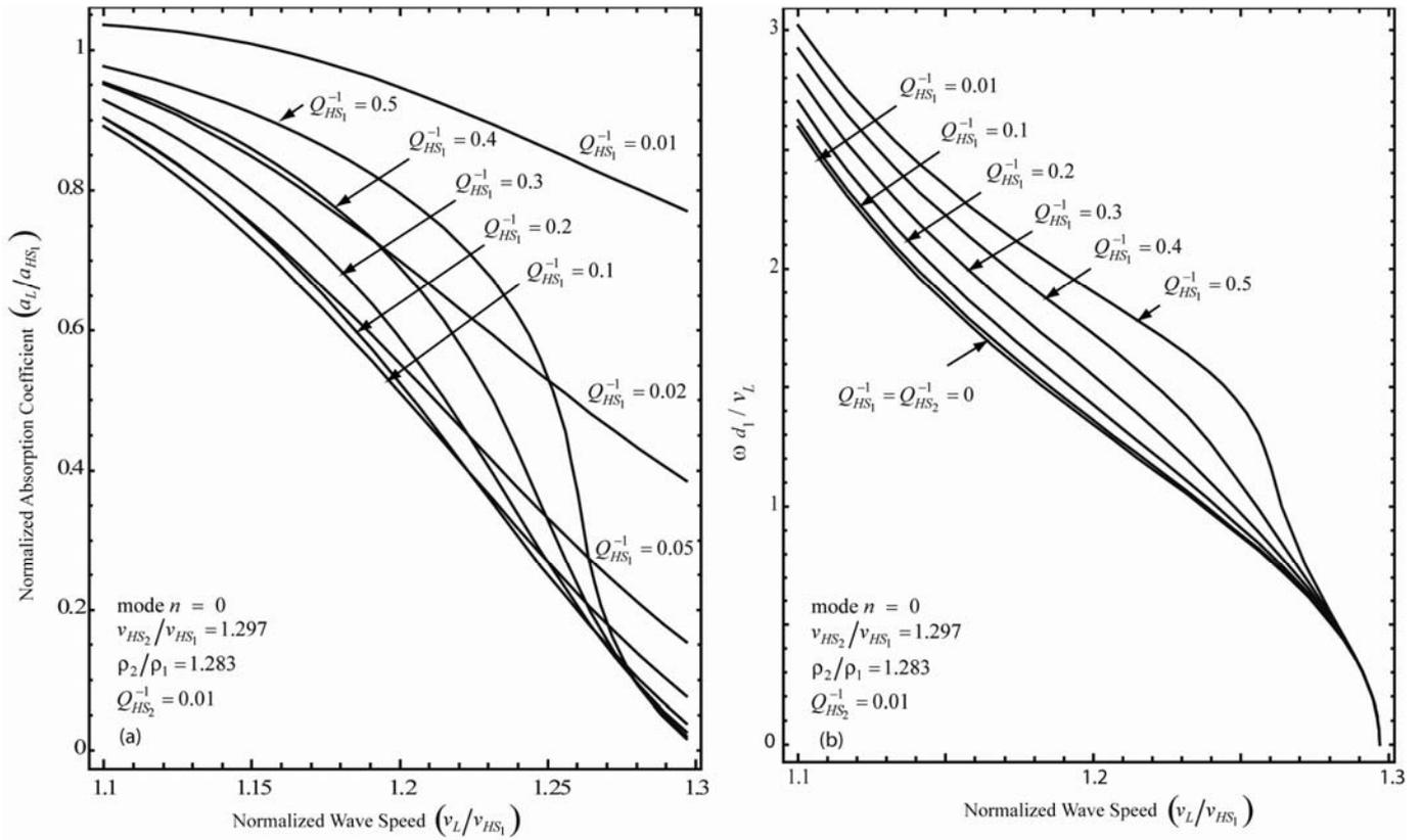
**Figure (1.18).** (a) Normalized absorption coefficient and (b)  $\omega d_1/v_L$  versus normalized wave speed for the fundamental mode of a Love-Type surface wave in viscoelastic media with material parameters as indicated.
