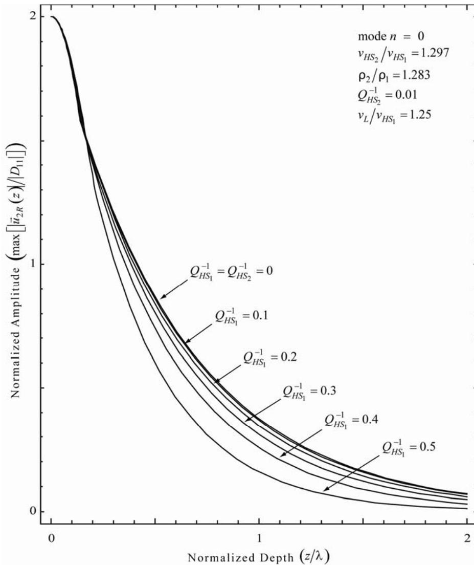
**Figure (1.19).** Normalized amplitude distribution for the fundamental mode of a Love-Type surface wave in viscoelastic media with material parameters as indicated.
