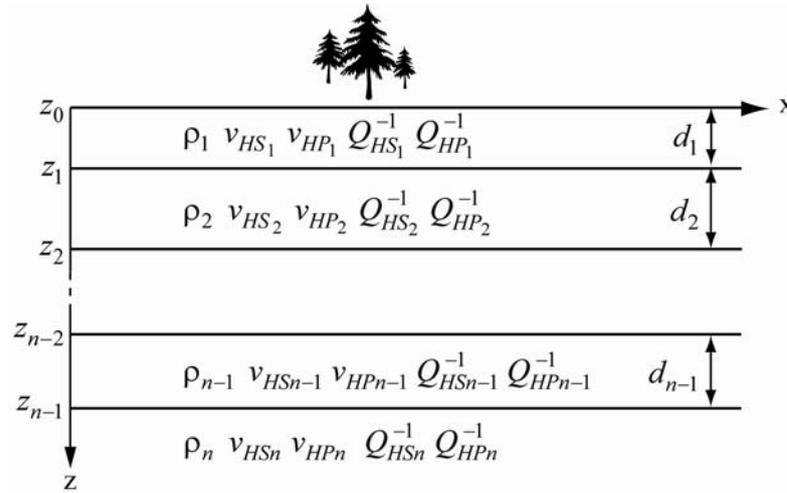
**Figure** (1.1). Diagram illustrating notation for the problem of a Love-Type Surface wave on multiple layered viscoelastic media.
