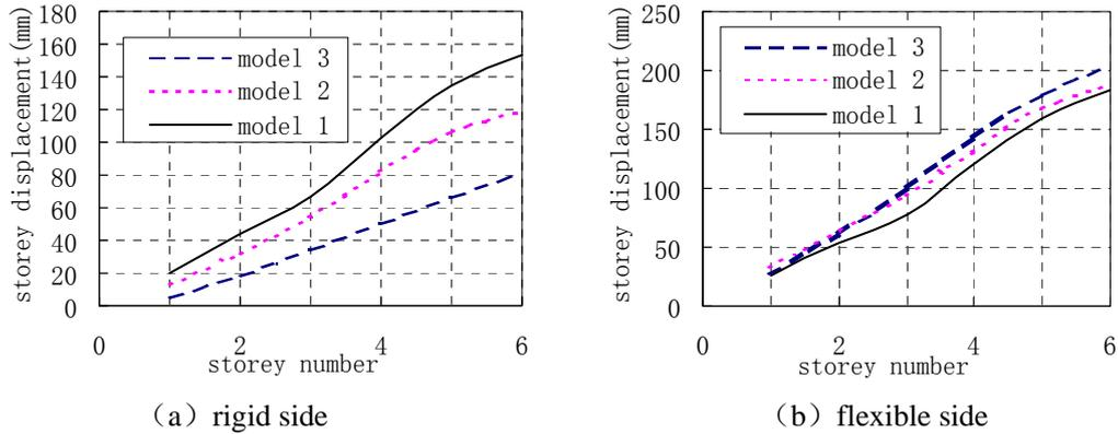
Figure 3 Model 1~3's maximum storey displacement in major earthquake, Y-direction
