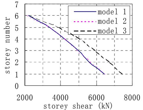
Figure 7 Storey shear force
