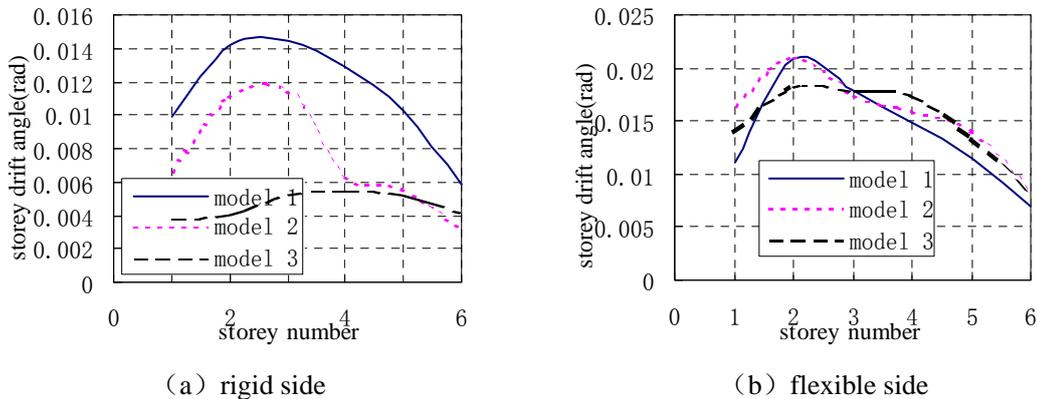
Fig. 4 Model 1~3's maximum storey drift angle in major earthquake, Y-direction
