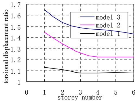
Fig. 6 maximum torsional displacement ratio
