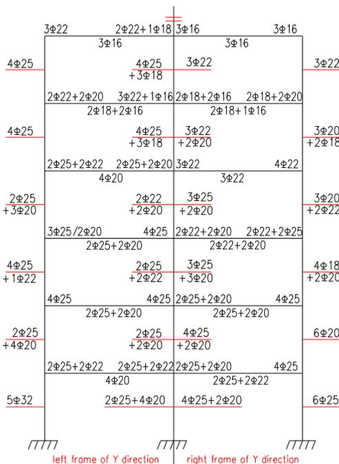
Fig. 1 Frame sectional reinforcement of model 3
