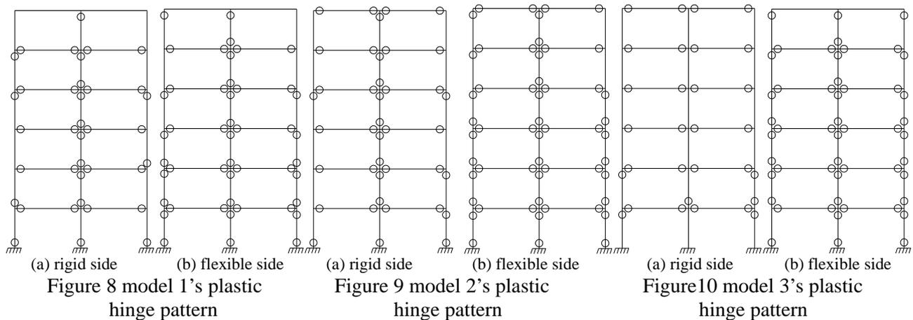
Figure 8 model 1's plastic hinge pattern
