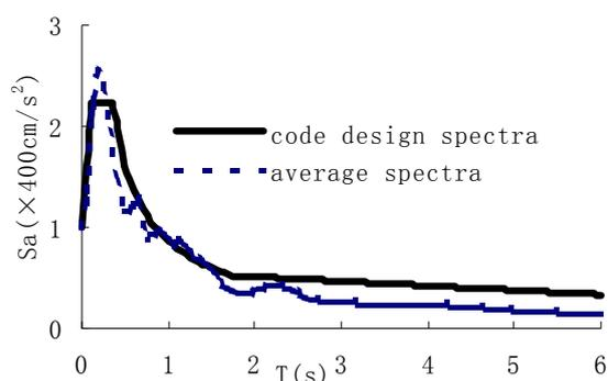
Figure 2 major quake spectrum against code spectrum
