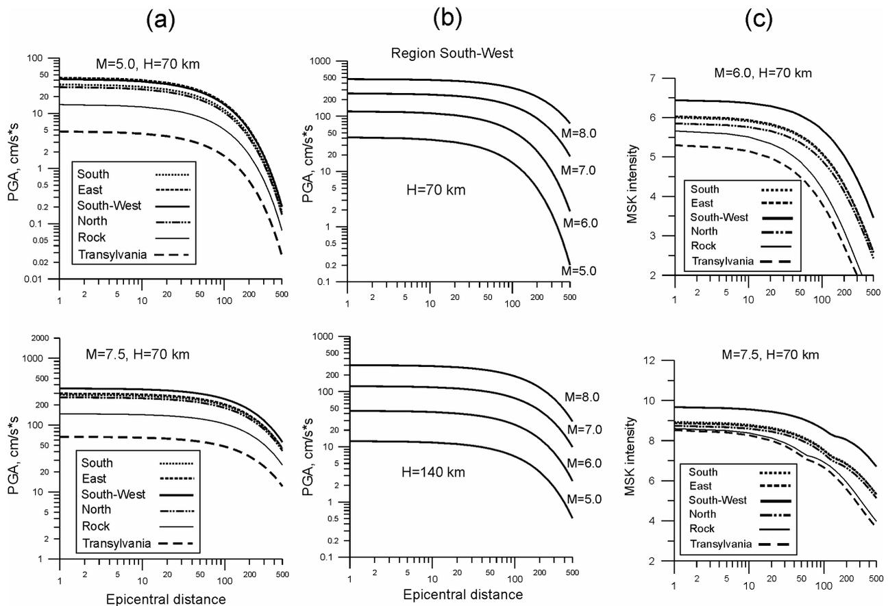
Figure 6. Examples of the attenuation curves developed for Romania (Sokolov et al., 2008). Comparison of the modelled PGA (a, b) and MSK intensity (c) curves for various zones, magnitudes ( $M$ ), depth ( $H$ ), and epicentral distances.
