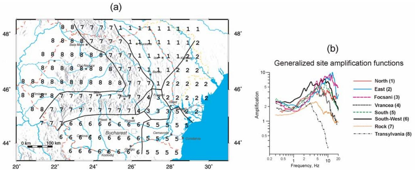
Figure 4. (a) Distribution of the generalized site amplification functions (regions) along the territory of Romania (see text for description of the numbers). (b) The generalized region-dependent site amplifications (mean amplitude values) including amplification for the “rock” category.
