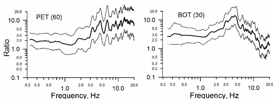
Figure 3. Examples of site amplification function (mean values and 1 standard deviation limits) for two soil sites - K2-stations: PET (epicentral area) and BOT (Bucharest). The numbers in parentheses show the number of used records.
