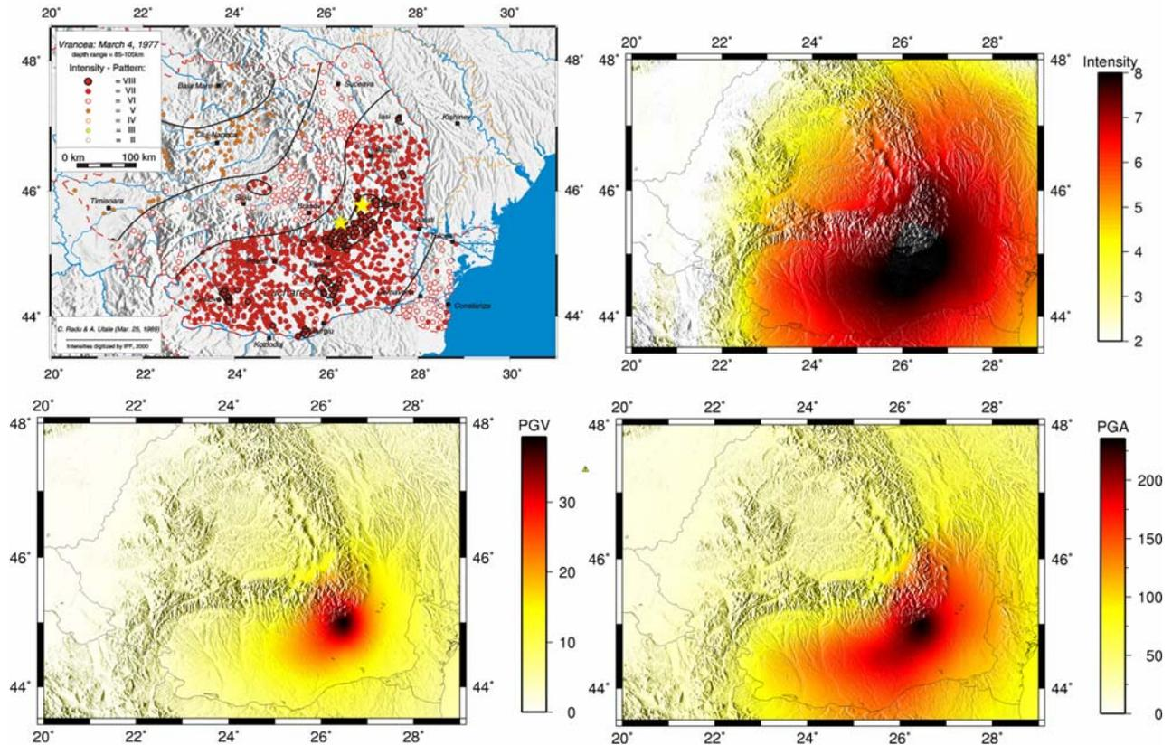
Figure 8. The observed macroseismic maps and the modelled distribution of ground motion parameters (MSK intensity, Peak Ground Acceleration and Peak Ground Velocity) for the earthquakes of March 4, 1977 ( $M_w$  7.4, depth 95 km).
