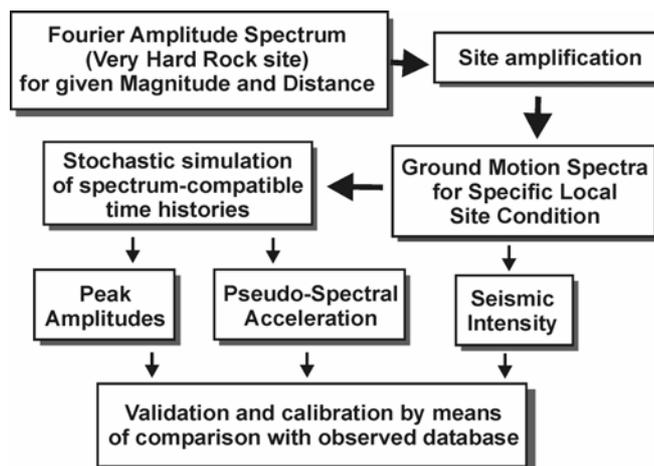
Figure 5. Scheme of evaluation of the ground-motion attenuation models based on the Fourier amplitude spectra.
