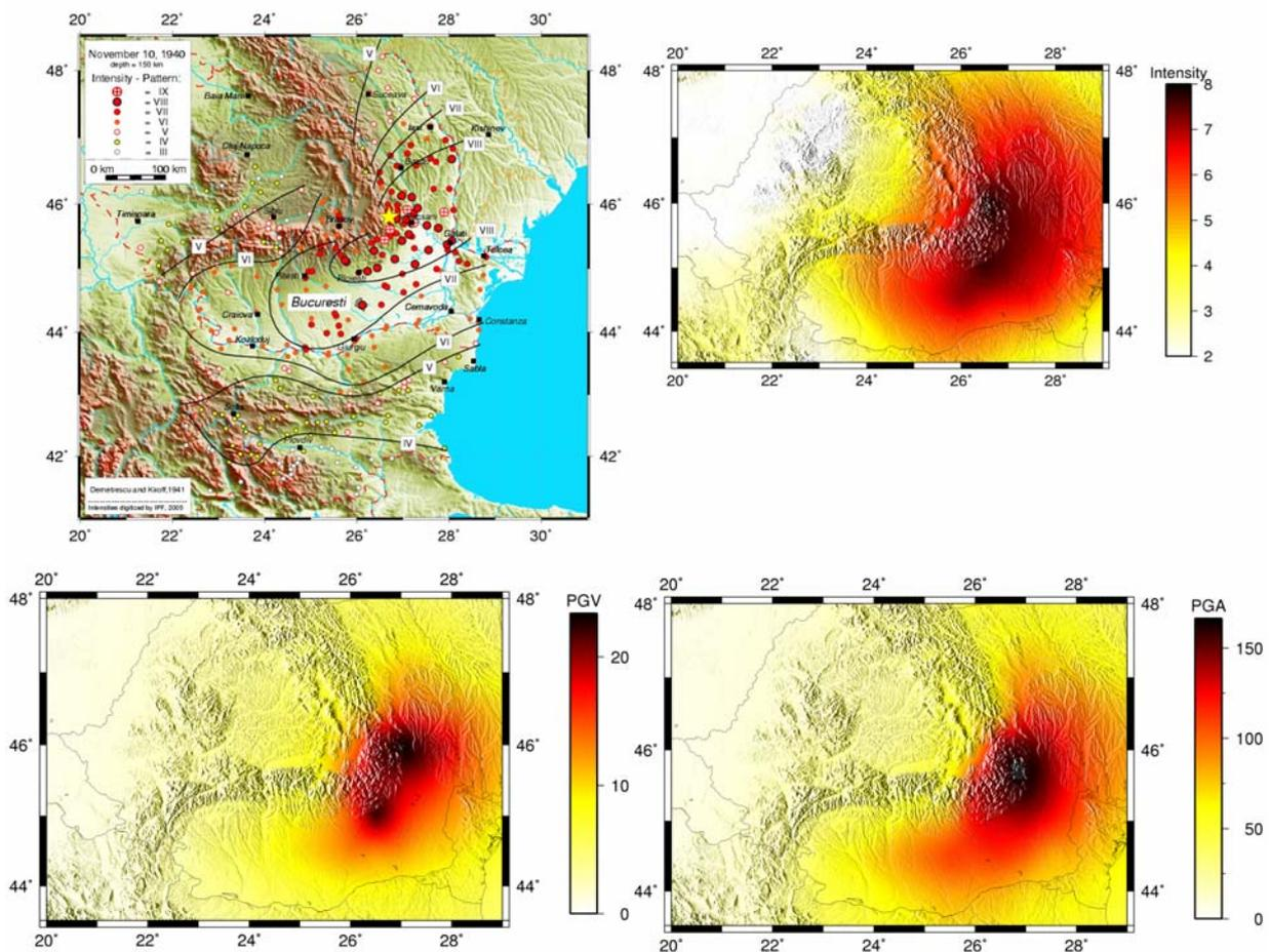
Figure 7. The observed macroseismic maps and the modelled distribution of ground motion parameters (MSK intensity, Peak Ground Acceleration and Peak Ground Velocity) for the earthquake of November 10, 1940 ( $M_w$  7.7, depth 140 km).
