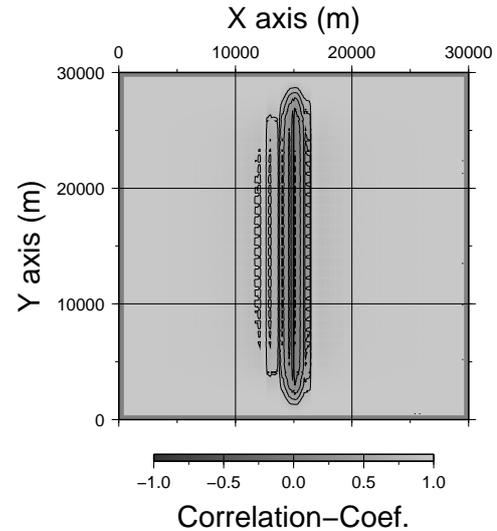
Figure 2 Distribution of correlation coefficients between gravity and magnetic anomaly.
