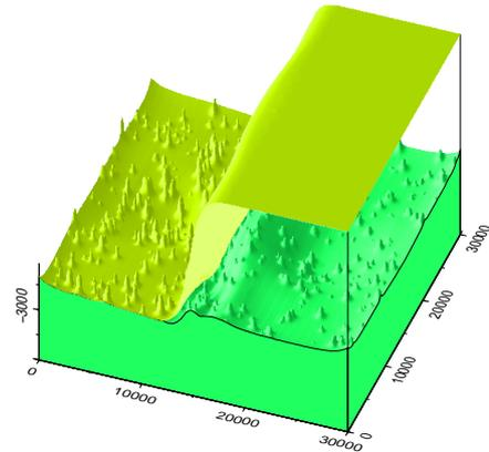
Figure 5 Estimated model of Figure 1 using the proposed method. The yellow and green surfaces are lower surfaces of the media with  $\Delta\rho = 0.15$  and  $\Delta\rho = 0.3$ , respectively.
