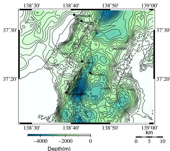
Figure 10 An estimated model of depth to the bedrock in this study.
