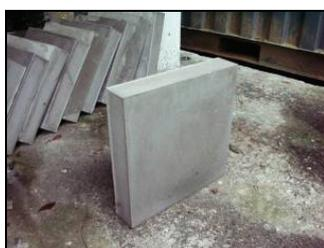
Figure 4 Cement mortar block
