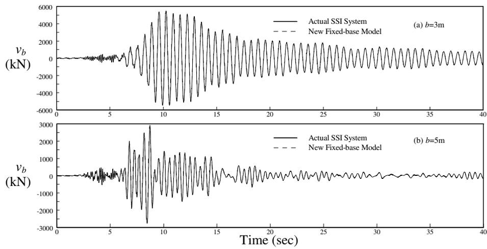
**Figure 4. Comparison of base shear to Loma Prieta earthquake**
