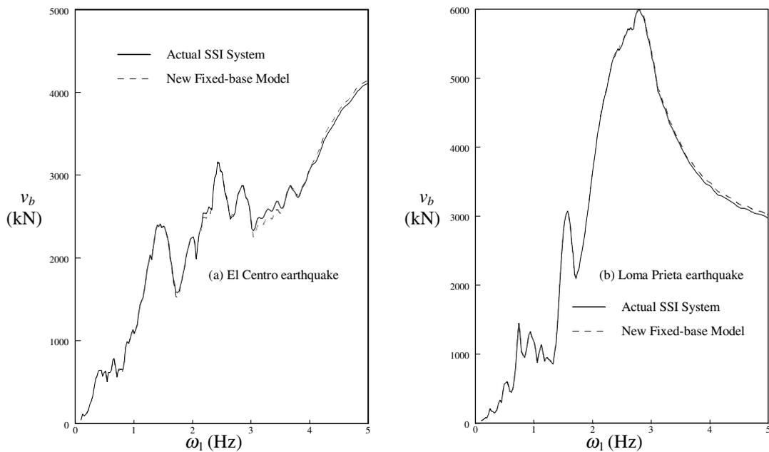
**Figure 5. Comparison of base shear spectrum to different earthquakes**
