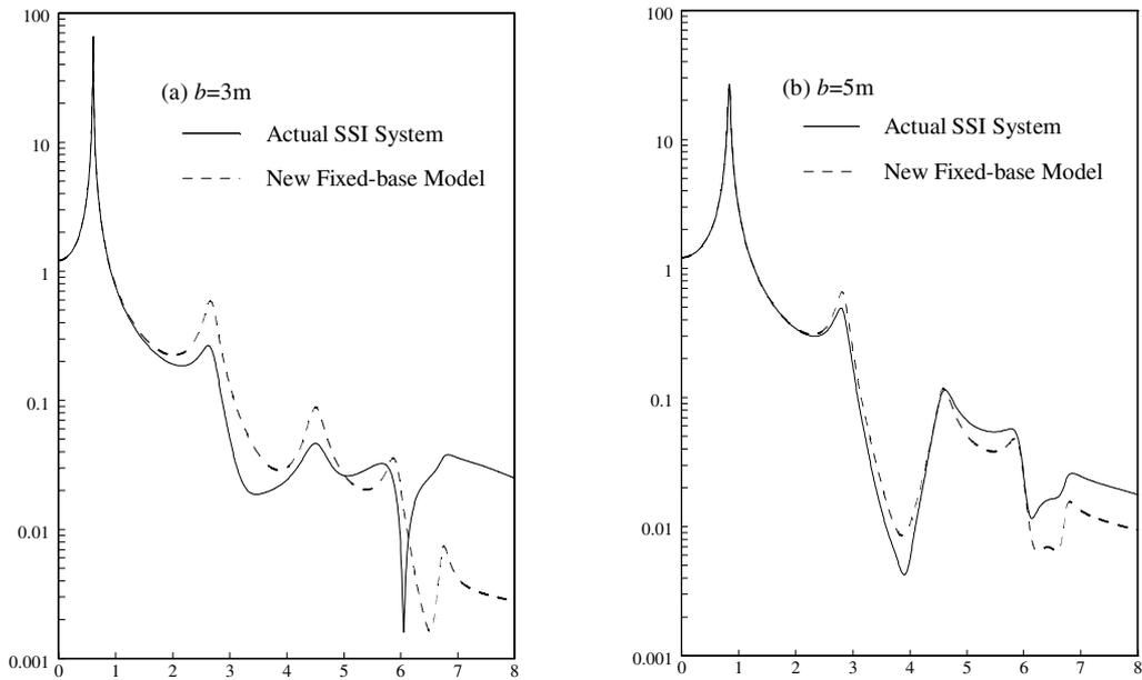
**Figure 2. Comparison of roof floor displacement in the frequency domain**
