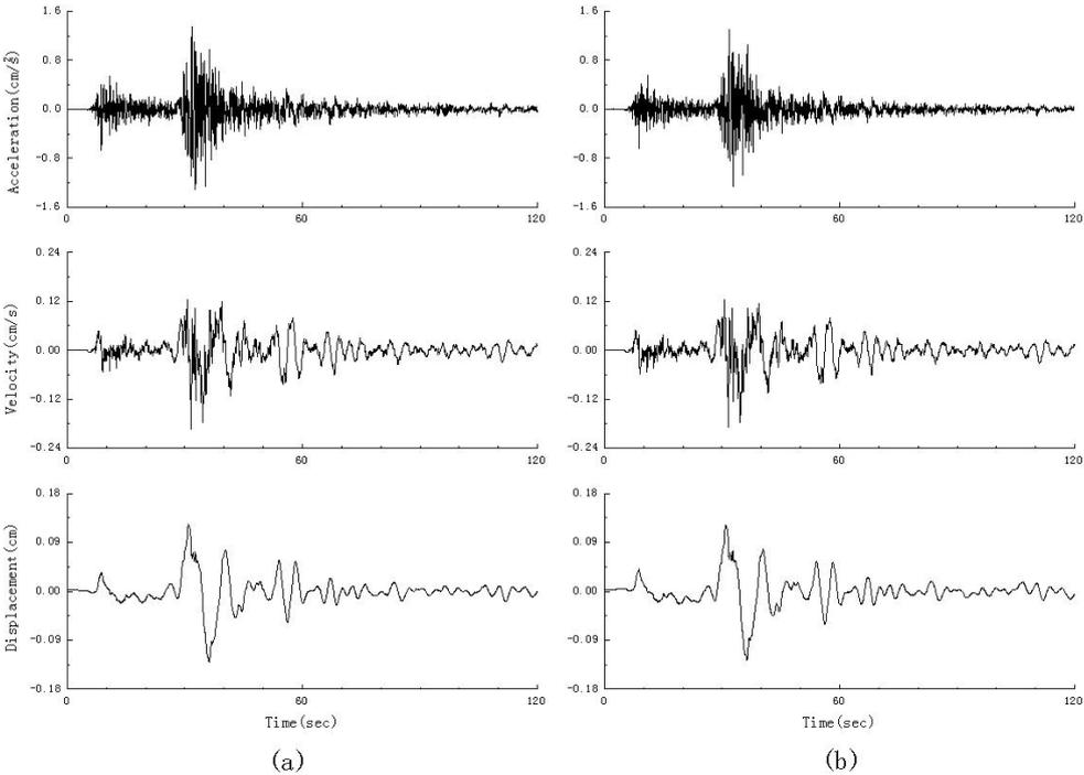
**Fig. 2 Recovered ground acceleration, velocity and displacement (from top to bottom, respectively) from VBB and LG of BJI station (a) VBB (b) LG**
