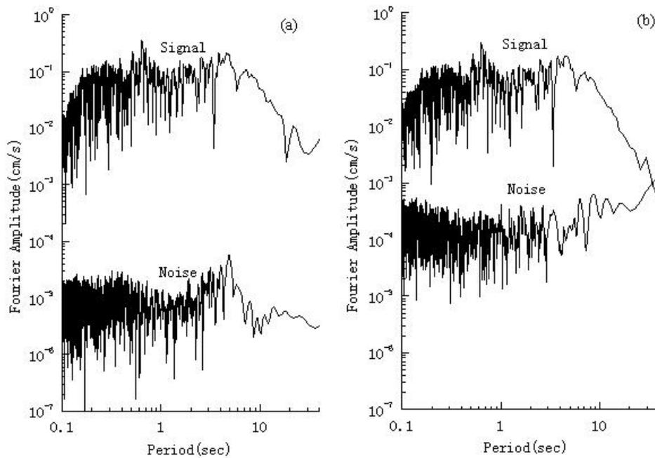
**Fig. 3 The comparisons of noise and seismic signals for VBB and LG (a) VBB (b) LG**
