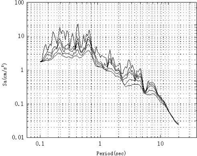
**Figure 5 The absolute acceleration response spectra from E-W component of VBB of BJI for Zhangbei earthquake. From top to bottom  $\zeta=0, 0.01, 0.02, 0.05, 0.10$**
