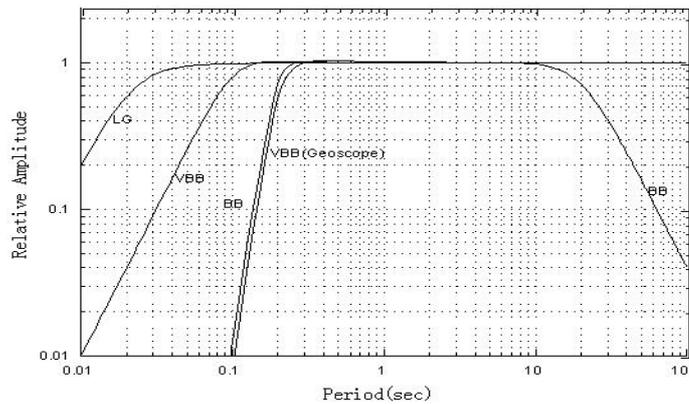
**Fig. 1 The frequency response of 4 seismometers. The LG is relative to acceleration and the others are relative to velocity.**
