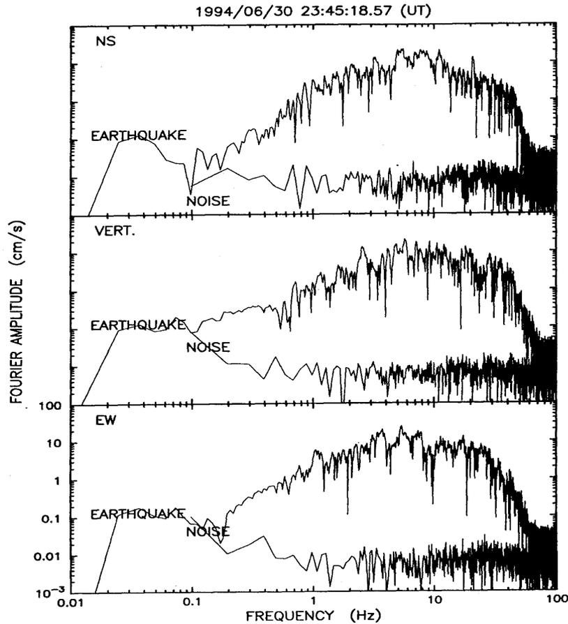
Fig. 4 The comparisons of noise and seismic signals for a typical SMART-2 data (Chiu (1997), Fig. 3)
