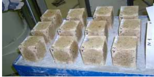
Figure 3: Compression tests on tuff elements: specimens set and test execution
