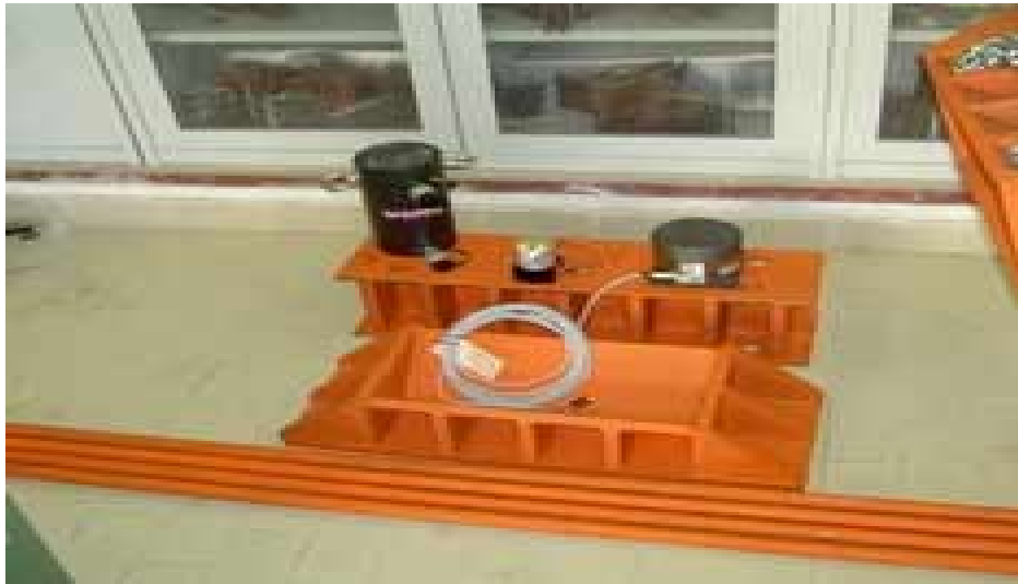
Figure 9: Measurement system: Oil jack, Wire Sensor and Load cell.
