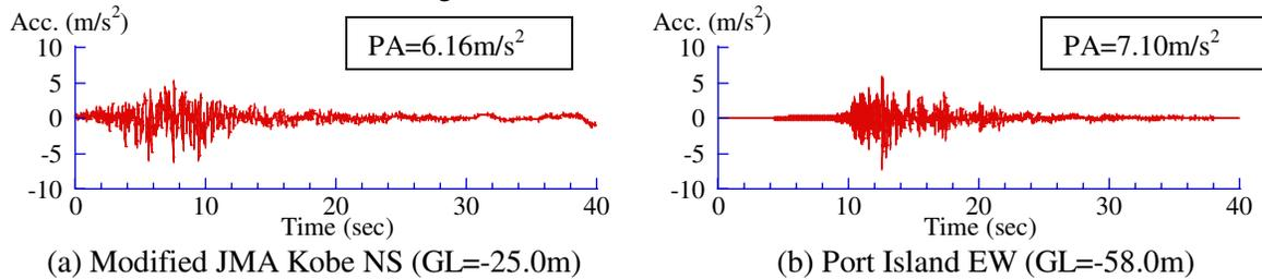
Figure 6 Input Earthquake Motion for the FEM Analysis (Bedrock Motion)
