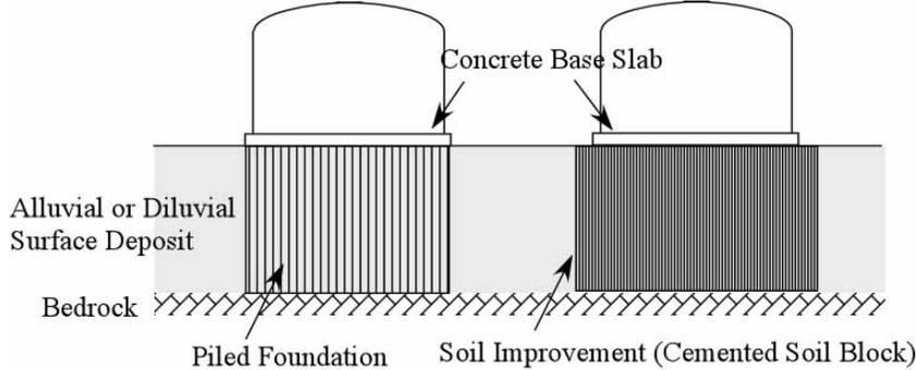
Figure 1 Piled Foundation and the “Seismic Action Control Foundation”
