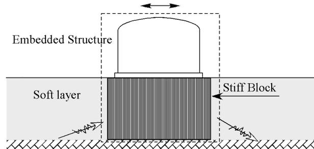
Figure 2 Schematic Mechanism of the Soil-Structure Interaction
