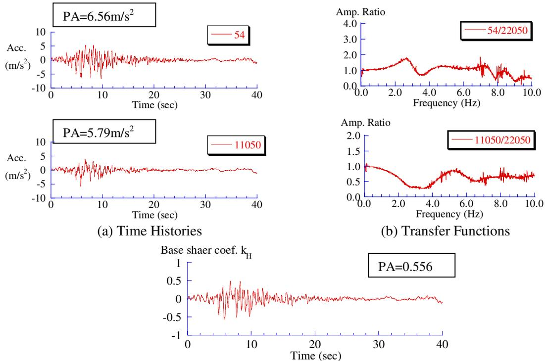
Figure 10 Typical Dynamic Responses of the Tank on the SACF (R1)
