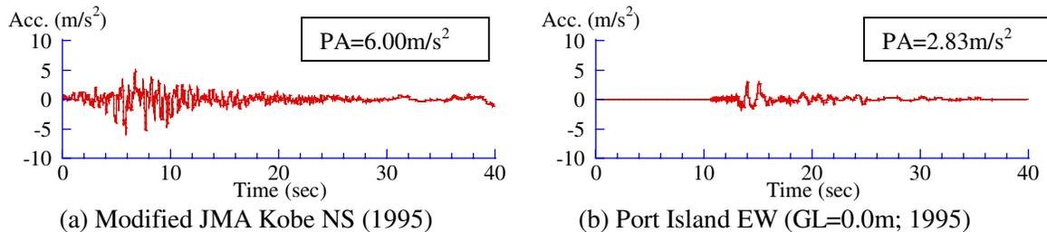
Figure 5 Ground Surface Motion
