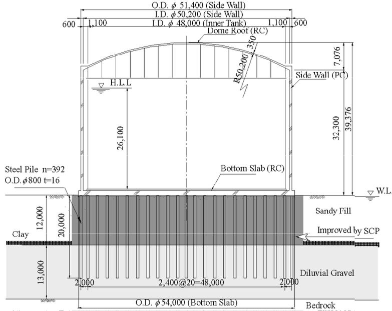
Figure 3 45,000m<sup>3</sup> LNG Storage Tank
