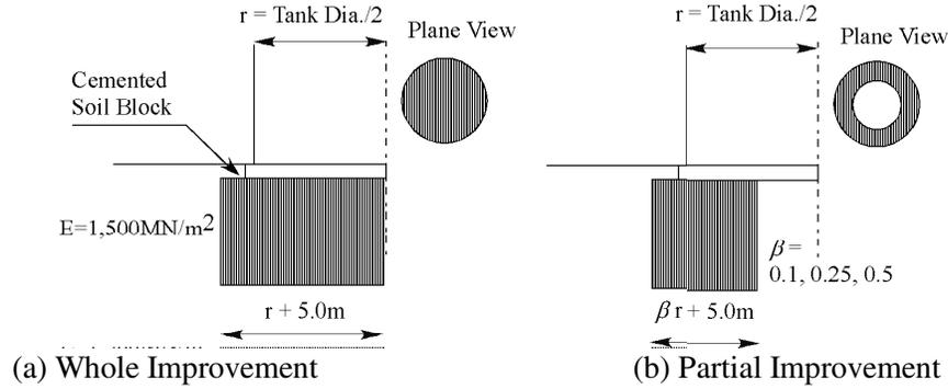
Figure 7 Area of the Cemented Soil Block
