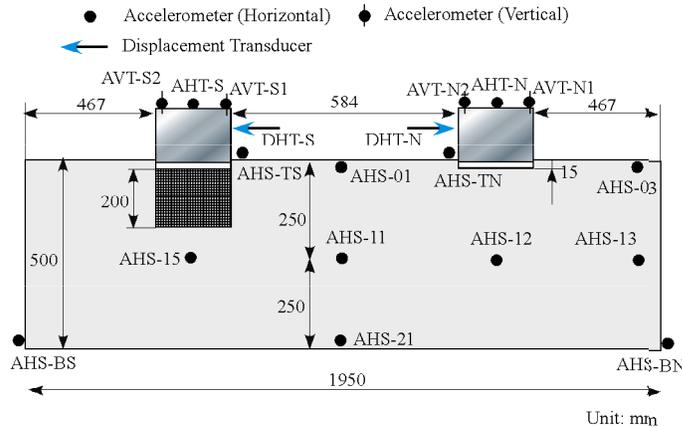
Figure 11 Model Setup for the Centrifuge Shaking Table Test for SACF (under 50g)
