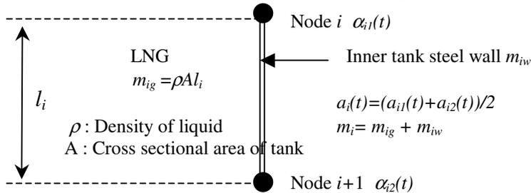
Figure 8 Mass of the Section and the Acceleration Time History of the Member
