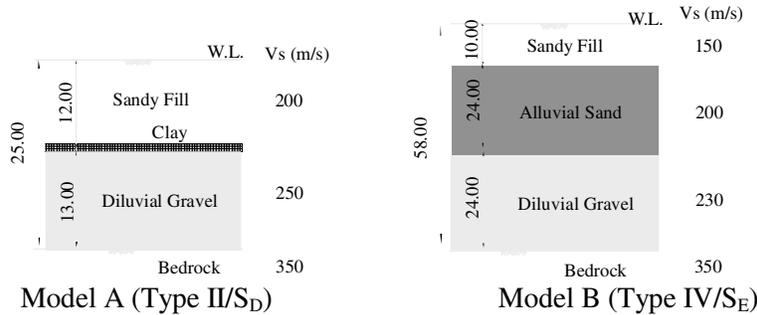
Figure 4 Soil Profiles of Subsurface Models
