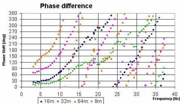
**Diagram 3.2.1.;** Phase shift between the sensors in the distances of 8, 16, 32, 64m and the reference sensor
