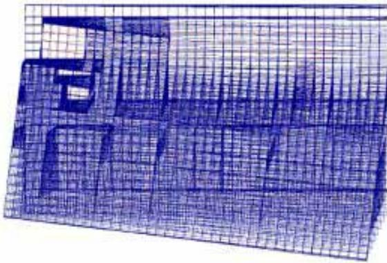
**Figure 4.1.4.1.;** calculated first Mode Shape
