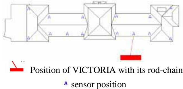
Figure 1.2.1.1.; position of sensors and VICTORIA
