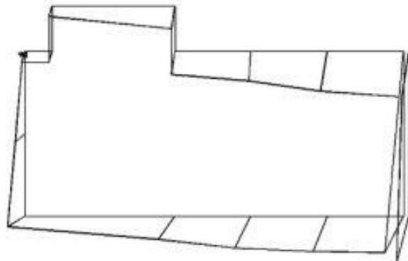
**Figure 4.1.4.2.;** measured first Mode Shape  $f=1.60$
