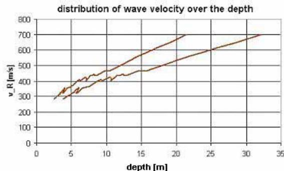
**Diagram 3.2.3.;** Rayleigh wave velocity in different soil depths
