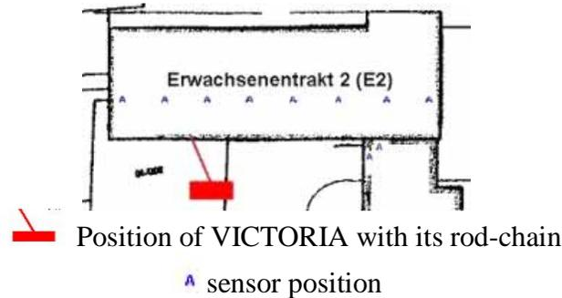
**Figure 1.1.3.1.;** position of sensors and VICTORIA
