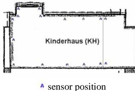
**Figure 1.1.4.1.;** positions of the sensors
