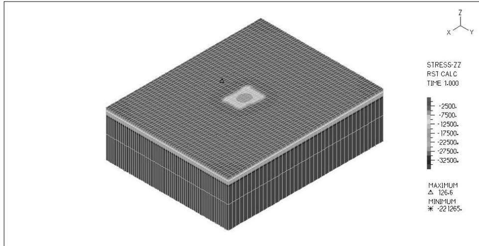
**Figure 4: Pressure under the foundation**
