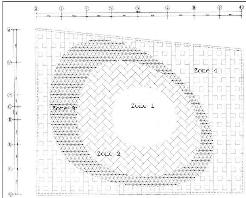
**Figure 6: Selected zones of  $K_s$  under the foundation**
