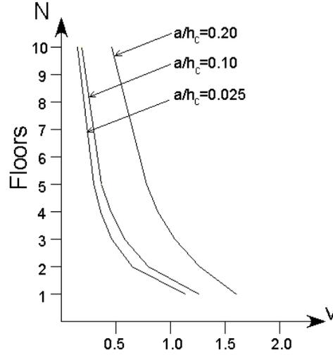
**Figure 3. Variation of coefficient  $v$  versus the increase of number of stories and of ratio  $a/h_c$**
