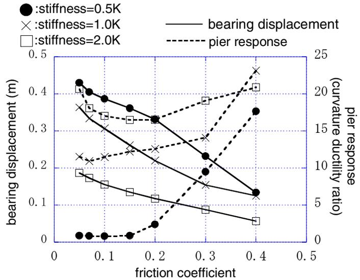
**Figure 9. Result of Analysis paying Attention to the Stiffness of Rubber Bearings and the Friction Coefficient of Sliding Bearings**
