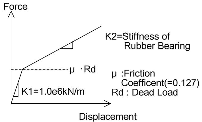
Figure 6. Simple Bilinear Model of Isolation System
