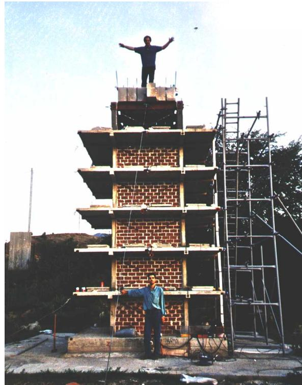
Photo1. 5<sup>th</sup> –story structure with masonry infills.
