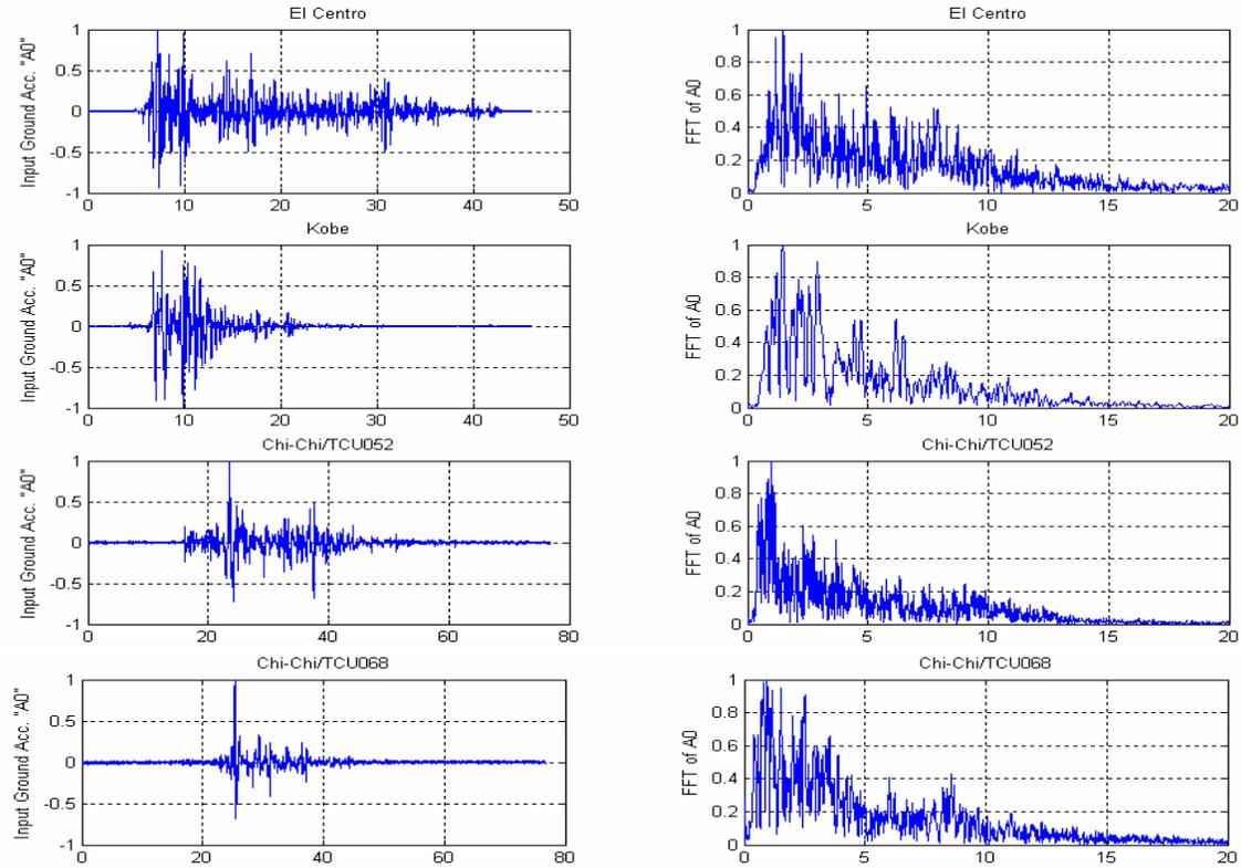
**Figure 7: Ground acceleration time histories (left) and their fast Fourier transforms (right) of the four earthquake records used in the shaking table test.**
