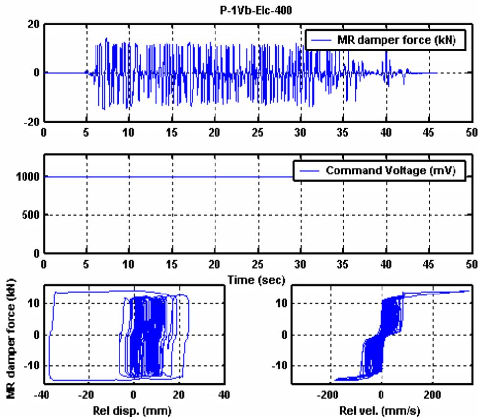
**Figure 11: Time history responses of the MR damper force (upper plot), command voltage (middle plot) and the hysteresis loops (lower left plot), force/velocity relationship of the MR damper in the passive controlled (“P-1V”) base-isolation system under El Centro earthquake excitation (PGA=0.4g).**
