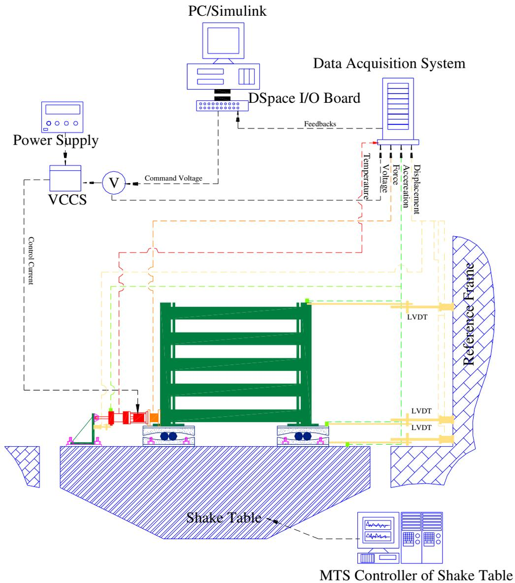
**Figure 4: Experimental setup of test structure.**
