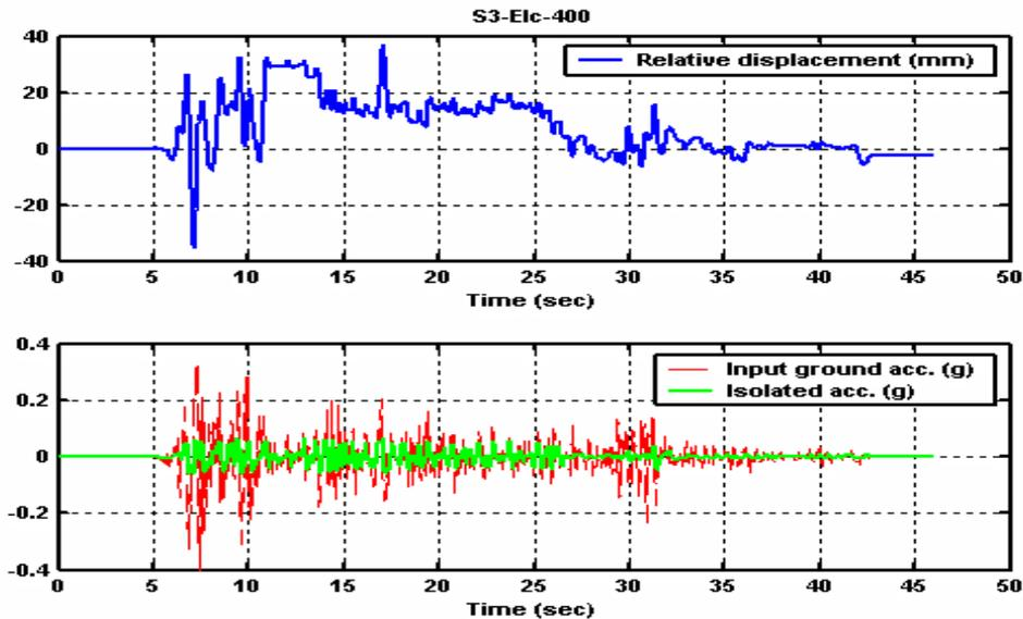
Figure 10: Time history responses of the relative displacement (upper plot), input ground acceleration and isolated acceleration (lower plot) of the semi-active controlled (“S3”) base-isolation system under El Centro earthquake excitation (PGA=0.4g).
