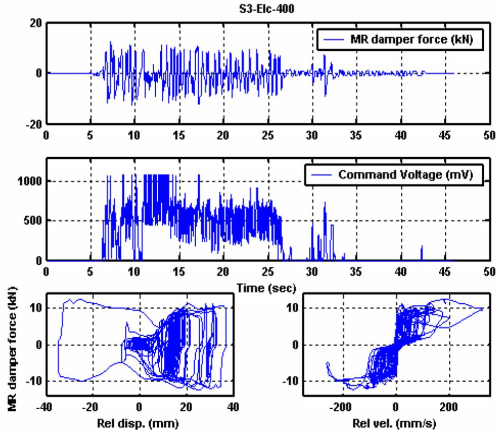
**Figure 12: Time history responses of the MR damper force (upper plot), command voltage (middle plot) and the hysteresis loops (lower left plot), force/velocity relationship of the MR damper in the semi-active controlled (“S3”) base-isolation system under El Centro earthquake excitation (PGA=0.4g).**
