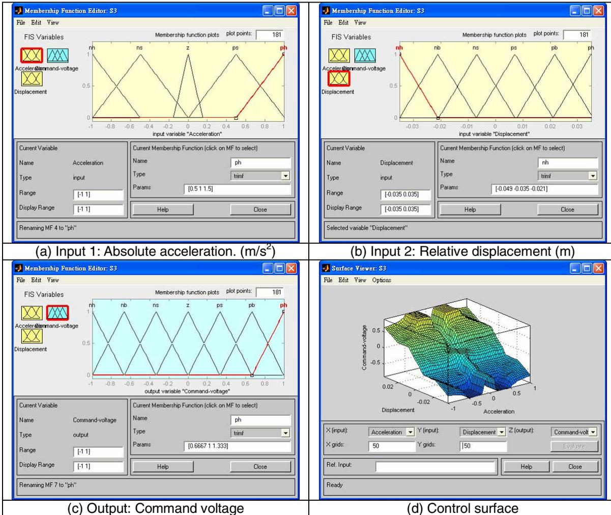
**Figure 3: Input and output membership functions of semi-active control surface “S3”.**
