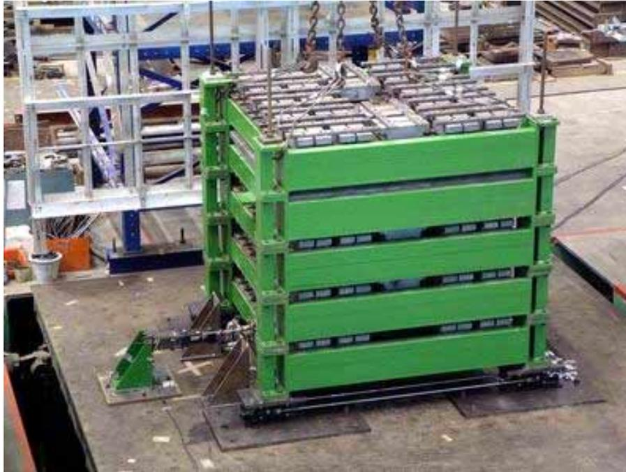
**Figure 6: Photo of the Semi-active controlled base-isolation system composed with the rolling pendulum system and MR damper.**
