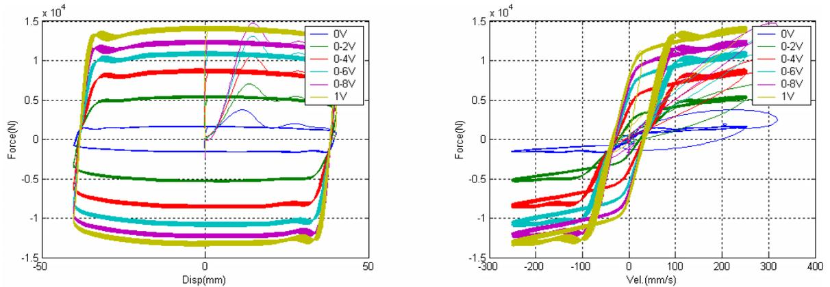
**Figure 1: Hysteresis loops (left plot) and damper force/velocity relationships (right plot) of the 20 kN MR damper with different command voltage inputs in the sinusoidal test (1Hz / 40mm).**
