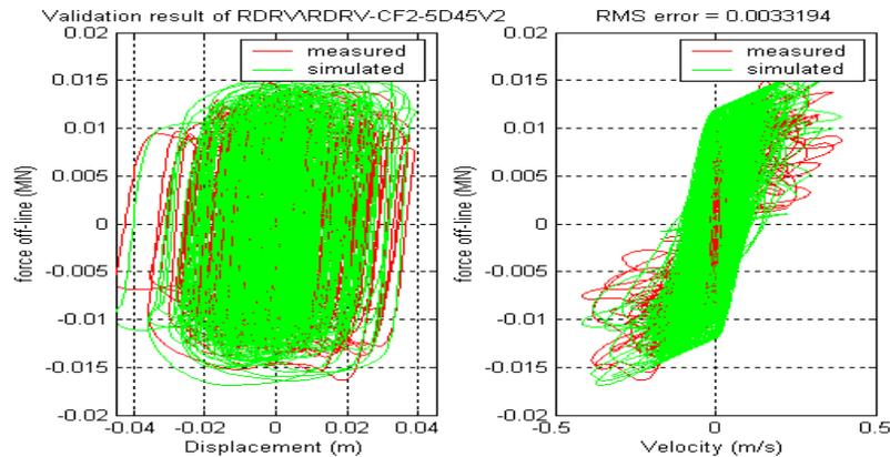
**Figure 2: Comparison of the measured and re-simulated hysteresis loops of the MR damper in the validation test.**
