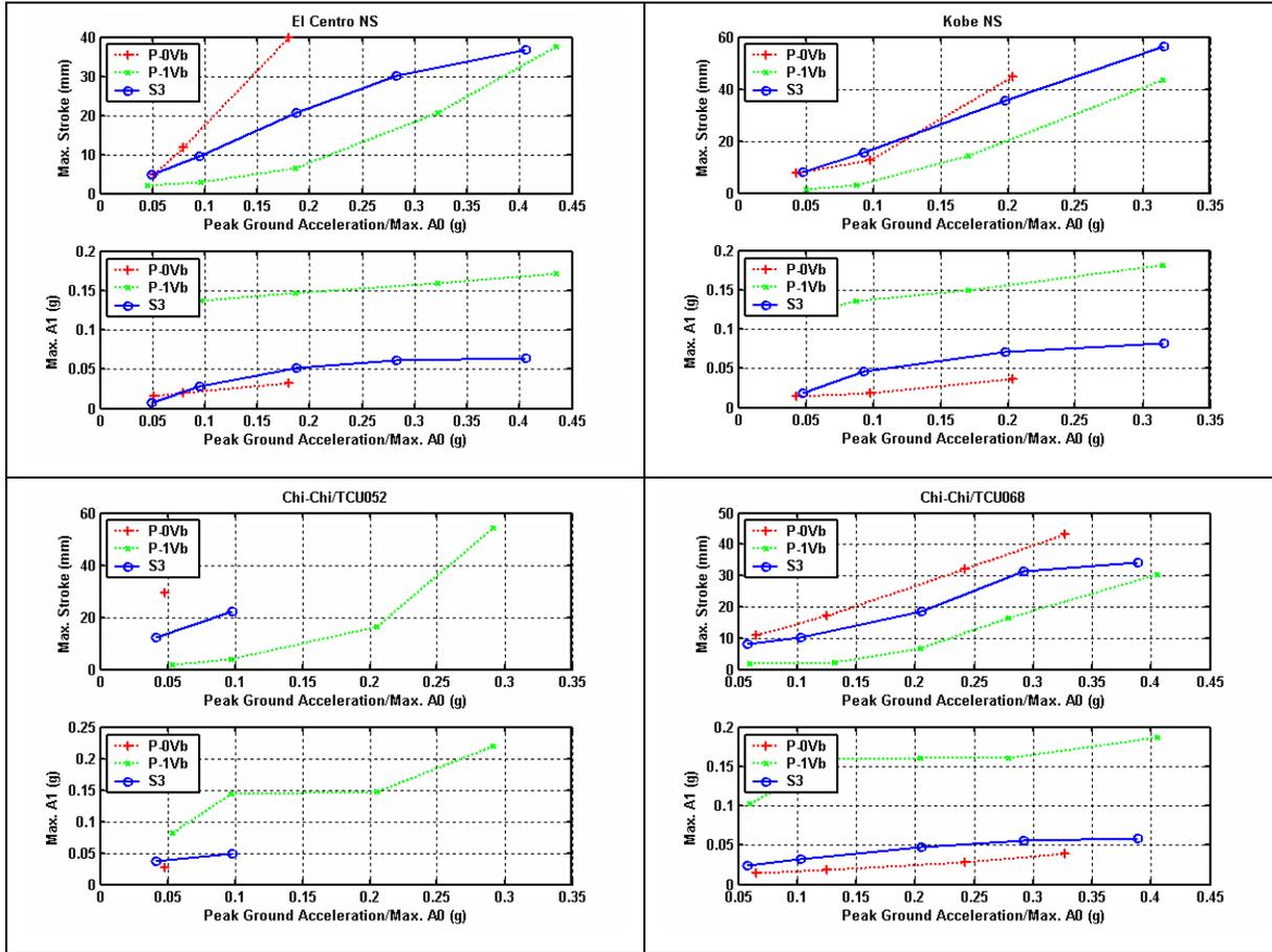
**Figure 8: Comparison of the maximum absolute acceleration (A1) and relative displacement (D1) of the hybrid controlled base-isolation system with different control cases.**
