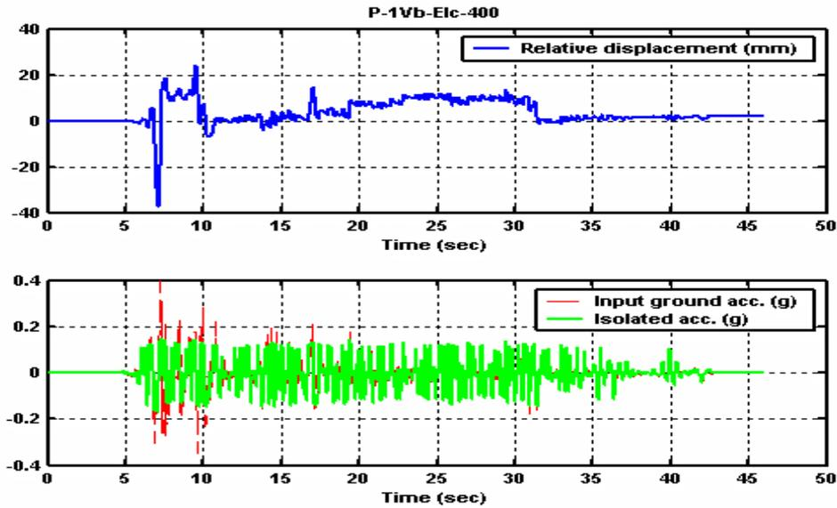
Figure 9: Time history responses of the relative displacement (upper plot), input ground acceleration and isolated acceleration (lower plot) of the passive-controlled (“P-1Vb”) base-isolation system under El Centro earthquake excitation (PGA=0.4g).
