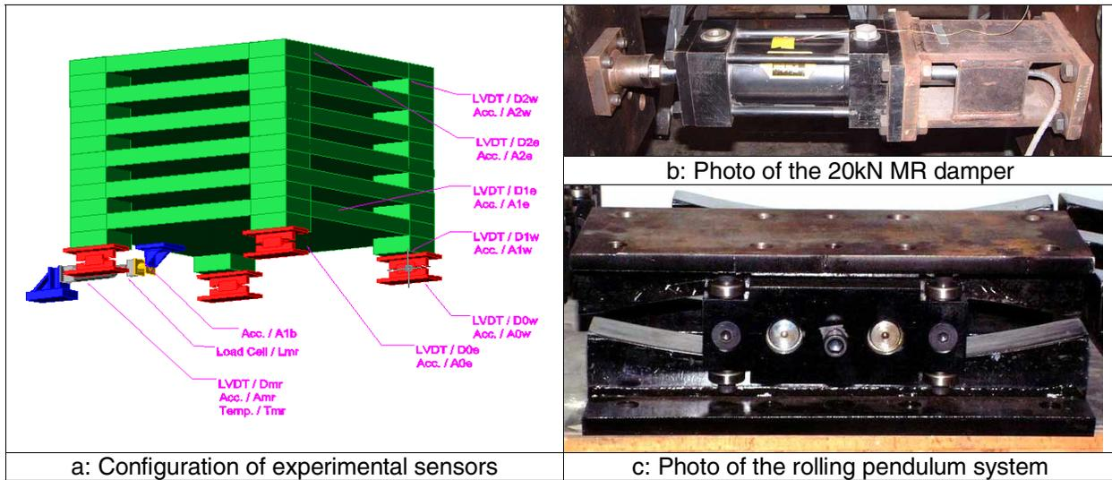
**Figure 5: Configuration of the experimental sensors and photo of the 20 kN MR damper and rolling pendulum system.**
