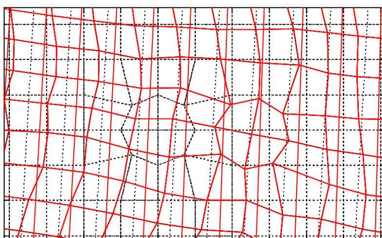
Fig. 6 Deformation of the Pile with Respect to the Liquefied Ground (Numerical Result)
