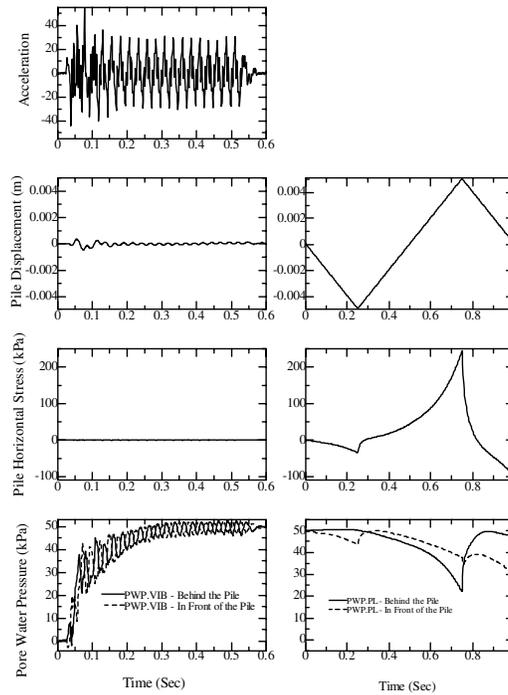
Figure 12. Numerical Analysis of Time Histories of Lateral Resistance and Displacement of Pile and Excess Pore Pressure around the Pile (Pile Loading Rate = 10 mm/sec)
