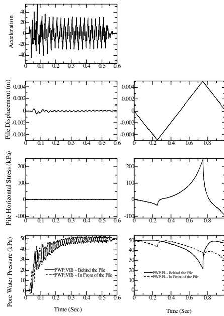
Figure 11. Numerical Analysis of Time Histories of Lateral Resistance and Displacement of Pile and Excess Pore Pressure around the Pile (Pile Loading Rate = 1 mm/sec)
