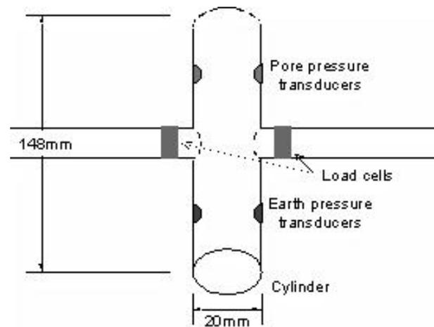
Fig. 3 Schematic Drawing of the Cylinder
