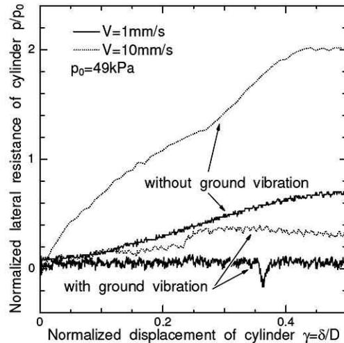
Figure 4. Normalized Lateral Resistance Against Normalized Lateral Displacement of Pile
