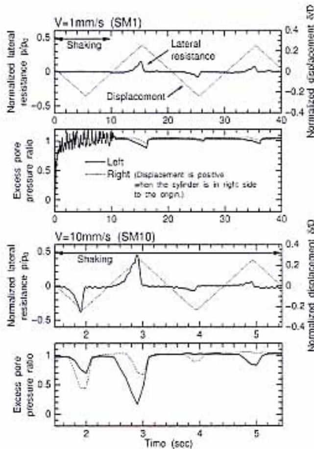
Figure 10 Time Histories of Lateral Resistance and Displacement of Pile and Excess Pore Pressure Around the Pile (SM1 and SM10)
