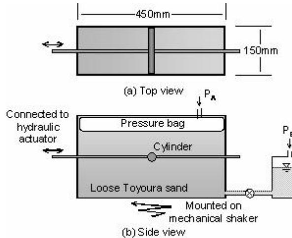
Fig. 2 Schematic Drawing of Model Container
