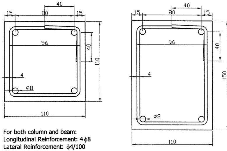
**Figure 2. Column and Beam Cross-Section**
