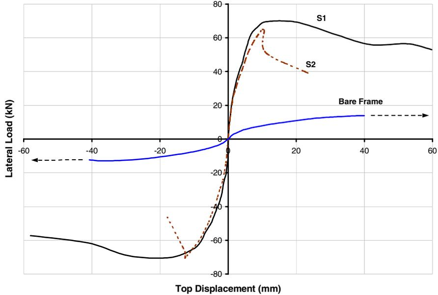
**Figure 7. Envelope Curves of the Specimens (Bare Frame is taken from Canbay et al. [4])**
