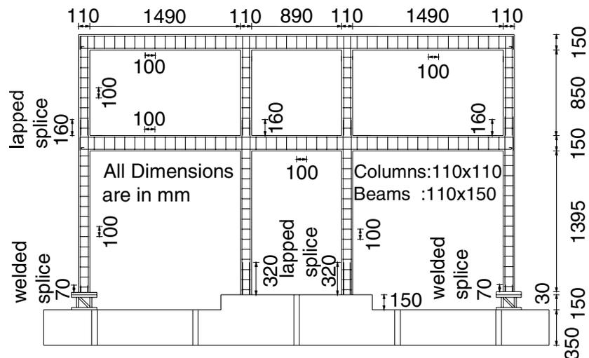
**Figure 1. Dimensions and Reinforcement Details of the Frame (Dimensions are in mm)**
