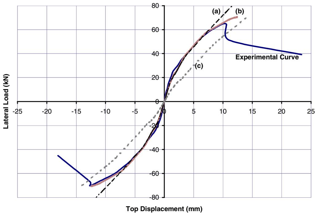
**Figure 15. Response Envelopes of Specimen S2**
