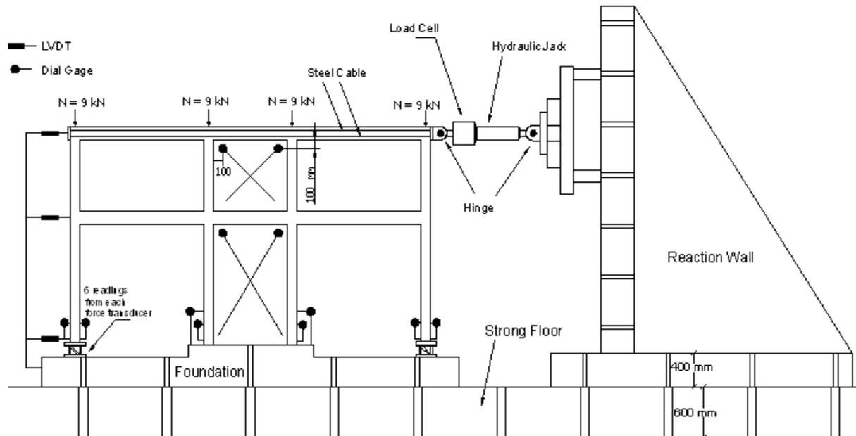
**Figure 6. Instrumentation and Test Setup**
