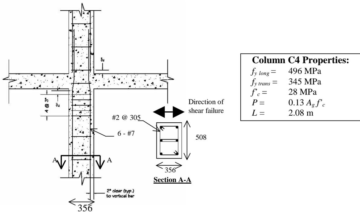
Figure 13. Details and assumed properties for fourth story column
