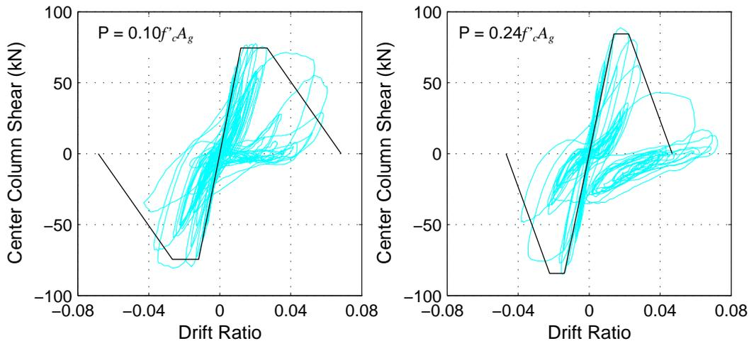
Figure 11. Center column hysteretic response compared with idealized backbone
