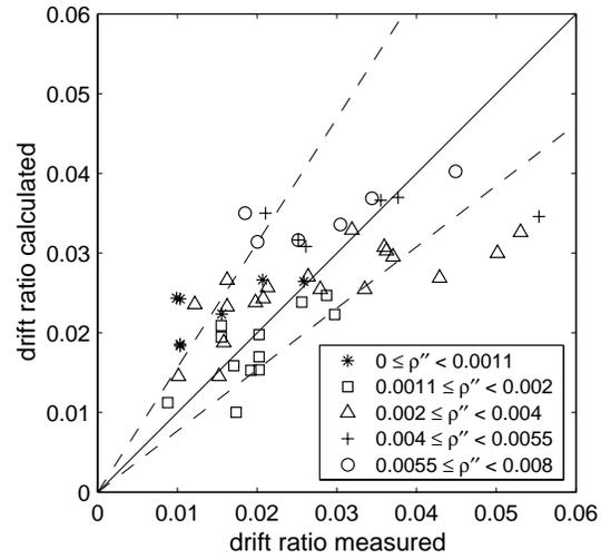
**Figure 5. Measured versus calculated drift at shear failure, Equation 6**
