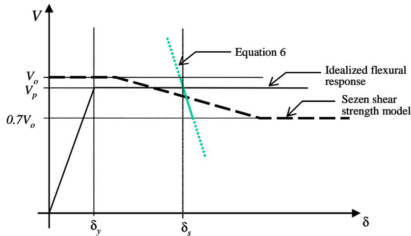
**Figure 8. Comparison of Sezen shear strength model and model for drift ratio at shear failure (Equation 6)**
