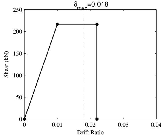
**Figure 15. Idealized backbone model for column C4.**
