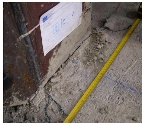
**Fig. 18. Failure in the concrete slab on an exterior joint of an exterior frame at a pga=1.4g**
