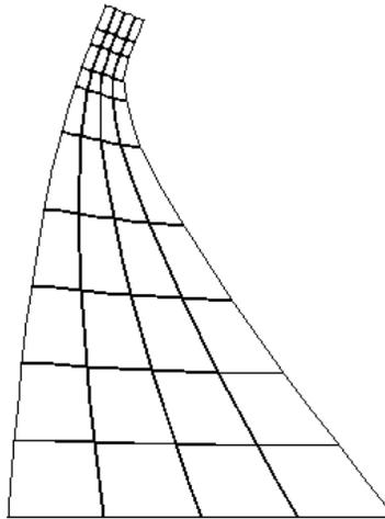
Figure 2. The first mode shape of the dam
