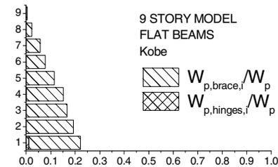
**Fig. 3: Distribution of the plastic strain energy in the 9-story models**
