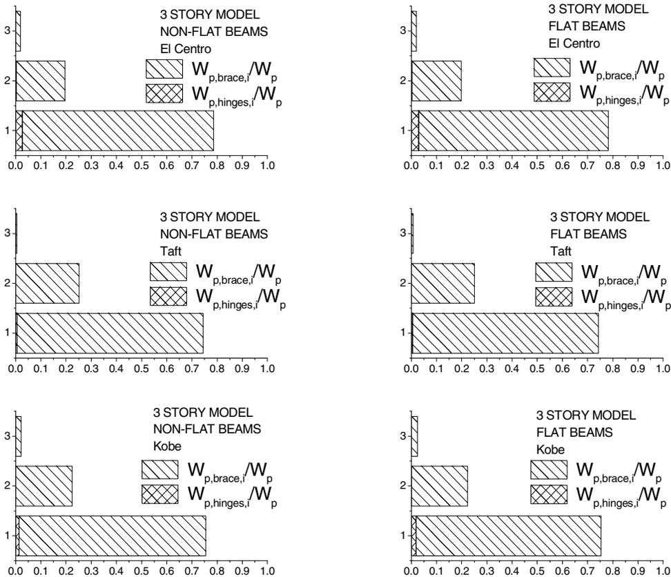
**Fig.1: Distribution of the plastic strain energy in the 3-story models**
