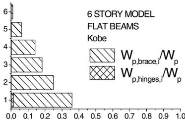
**Fig. 2: Distribution of the plastic strain energy in the 6-story models**
