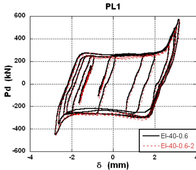
**Fig. 13 Effect of Excitation Frequency under Random Excitation (PL1)**
