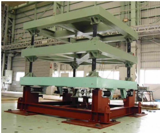
Figure 18 Test building model
