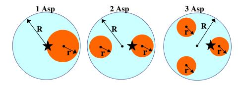
**Figure 1**. Circular asperity models for dynamic rupture simulation of sub-surface earthquakes. *R* and *r* are the radii of the circular fault and circular asperity respectively. The star represents the hypocenter.
