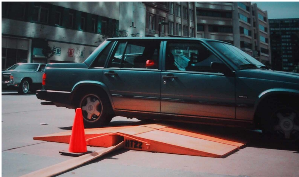
Figure 8. Use of Ramp Over A 5" Diameter Flex Hose
