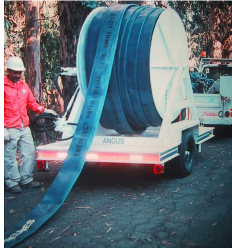
Figure 6. Alternate Deployment of Flex Hose
