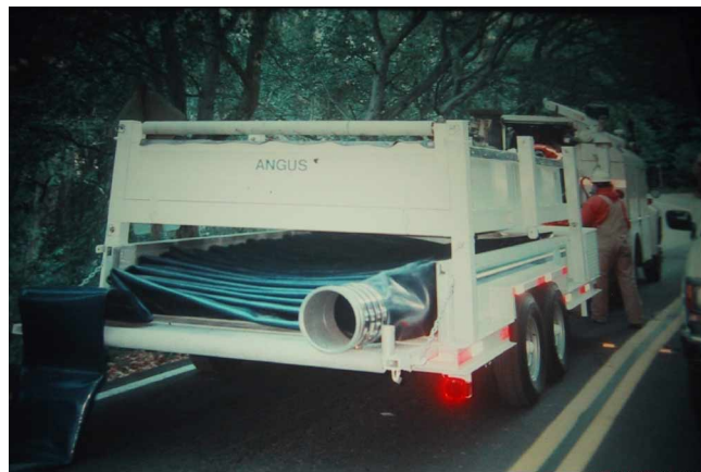
Figure 5. Deployment of Flex Hose
