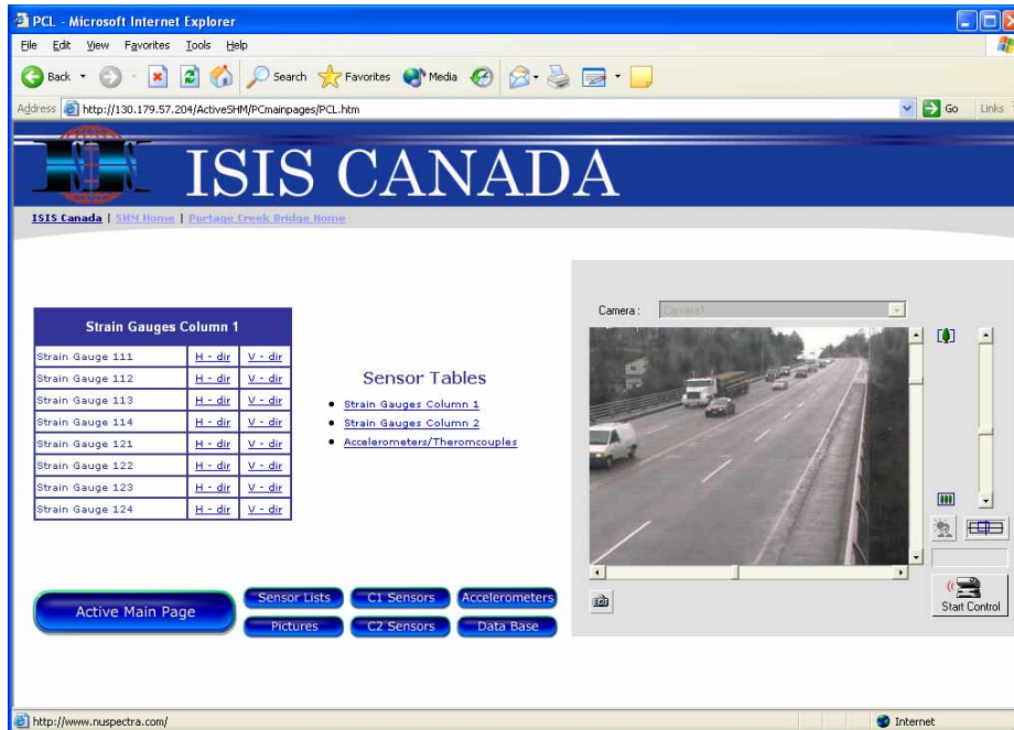
Fig. 8 Portage Creek Bridge SHM web page integrating sensing data and web camera
