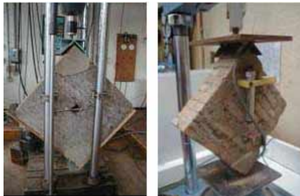
Figure 1. Diagonal tension test on real scale (left), and reduced scale wallettes (right).
