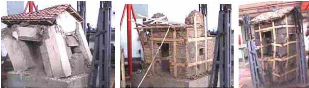
Figure 9. Failure- mechanism for 1:5 scale models tested on
