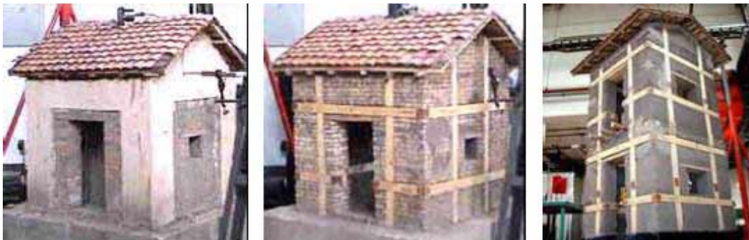
Figure 8. Reinforced models tested on vibratory table
