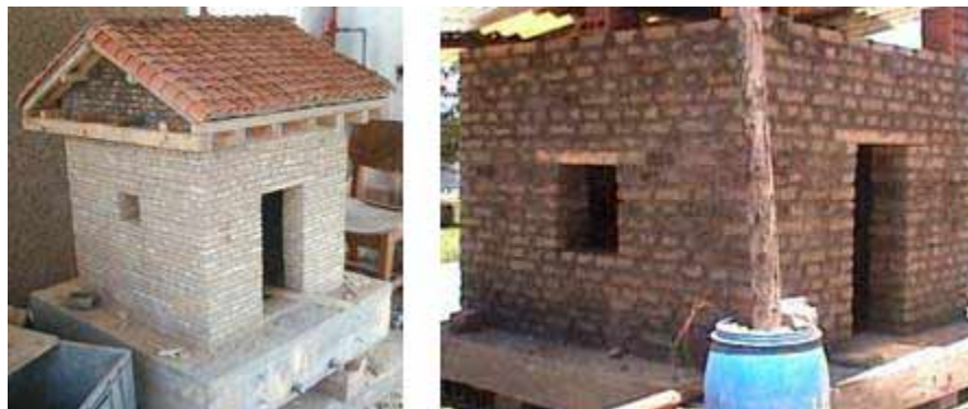
Figure 4. 1:5 scale models tested on shaking table and 1:1.5 scale models tested with applied cyclical loading
