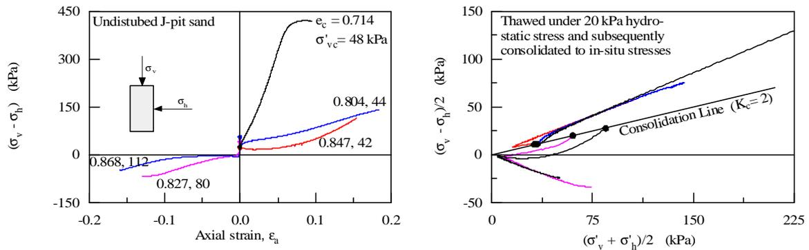
Figure 7: Undrained triaxial response of undisturbed J-pit (Syncrude) sand
