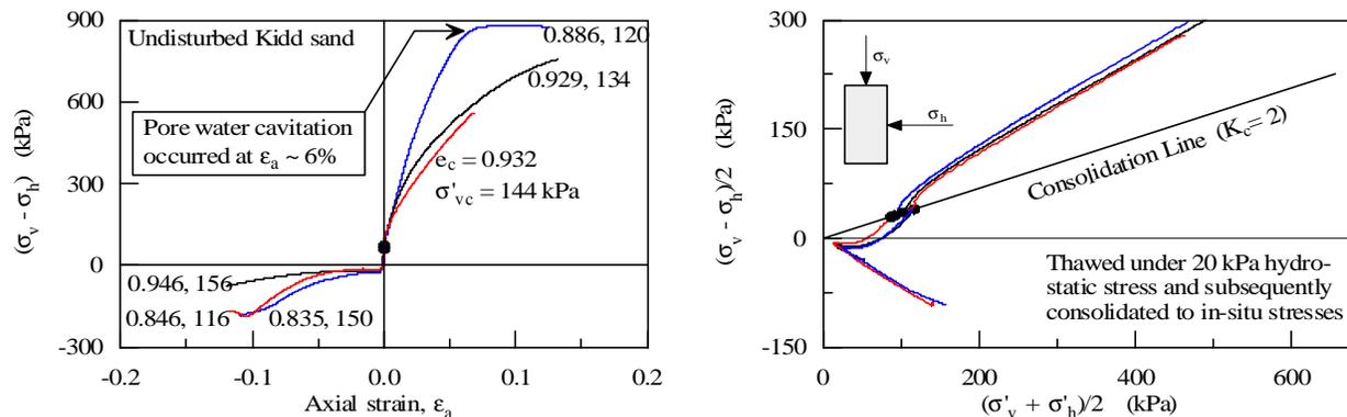
Figure 4: Undrained triaxial response of undisturbed Mildred Lake sand specimens
