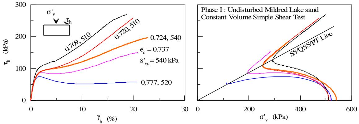
**Figure 8: Range of undrained simple shear response in undisturbed Mildred Lake sand**
