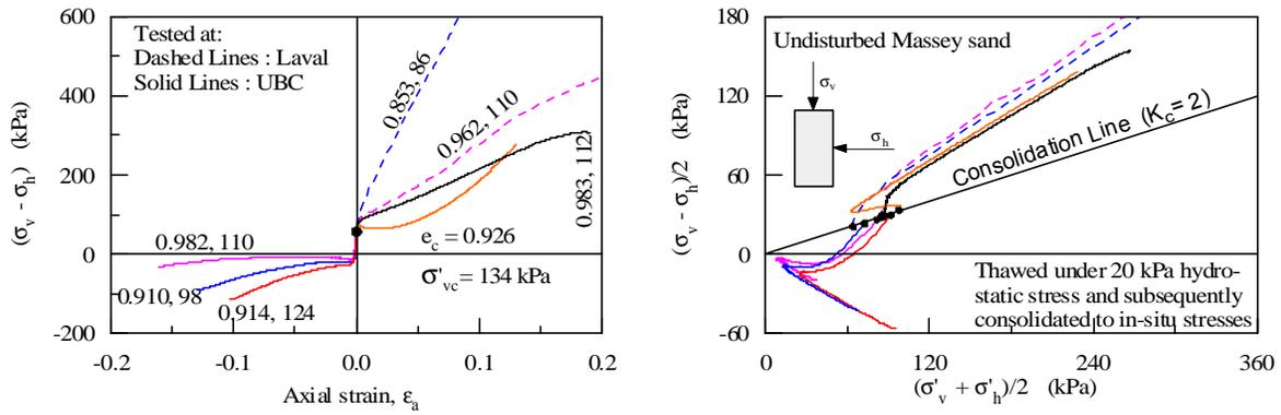
Figure 5: Undrained triaxial response of undisturbed Massey sand
