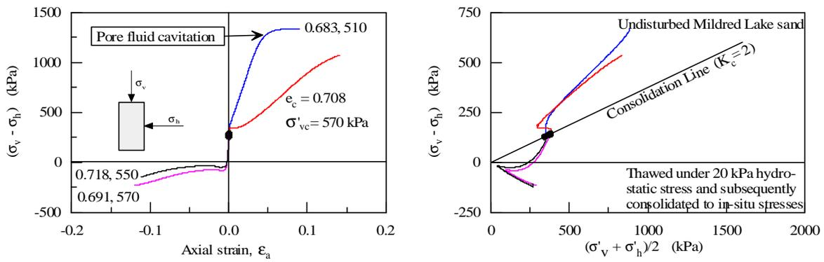
Figure 6: Undrained triaxial response of undisturbed Mildred Lake (Syncrude) sand
