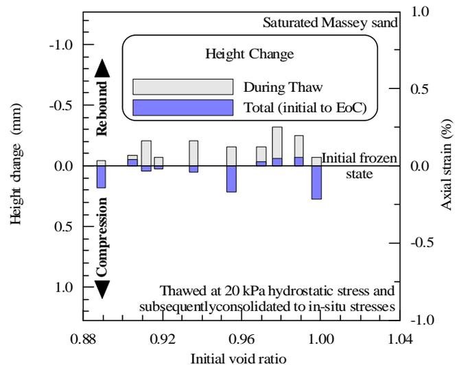
Figure 2: Height change during thaw and consolidation in saturated Massey sands
