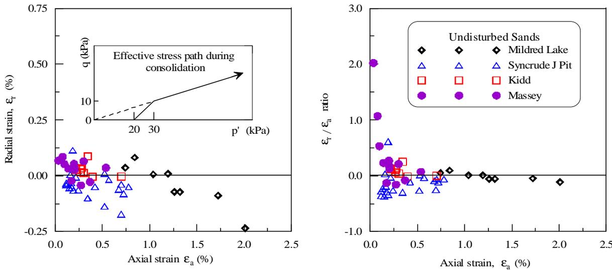
Figure 3: Axial and radial strain during reinstatement of in-situ stresses following thaw
