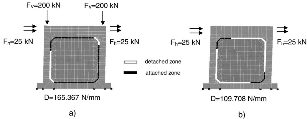
**Figure 4.** Some results of the preliminary FEM analysis: infill made before (a) and after (b) the application of vertical loads
