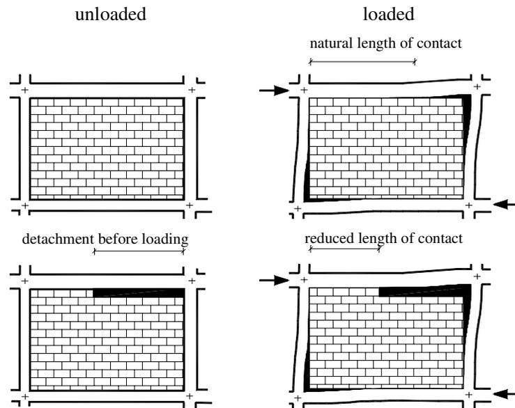
**Figure 6.** Control of the length of contact at the right upper corner
