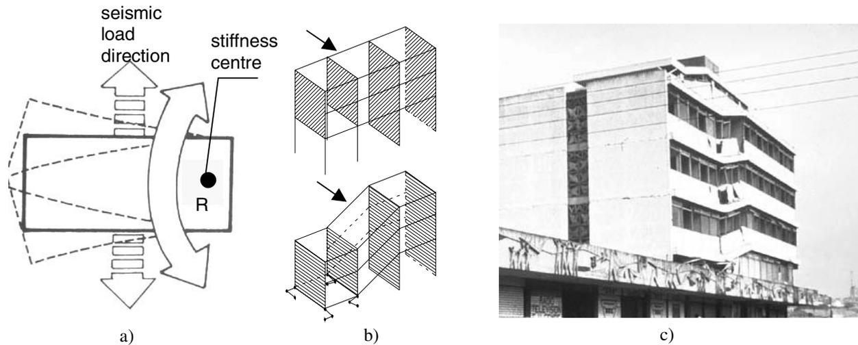
**Figure 1.** Effect of infills not uniformly distributed in plan: a) plan view: torsional effect ; b) axonometric view: scheme before and after collapse; c) building which has collapsed under seismic action
