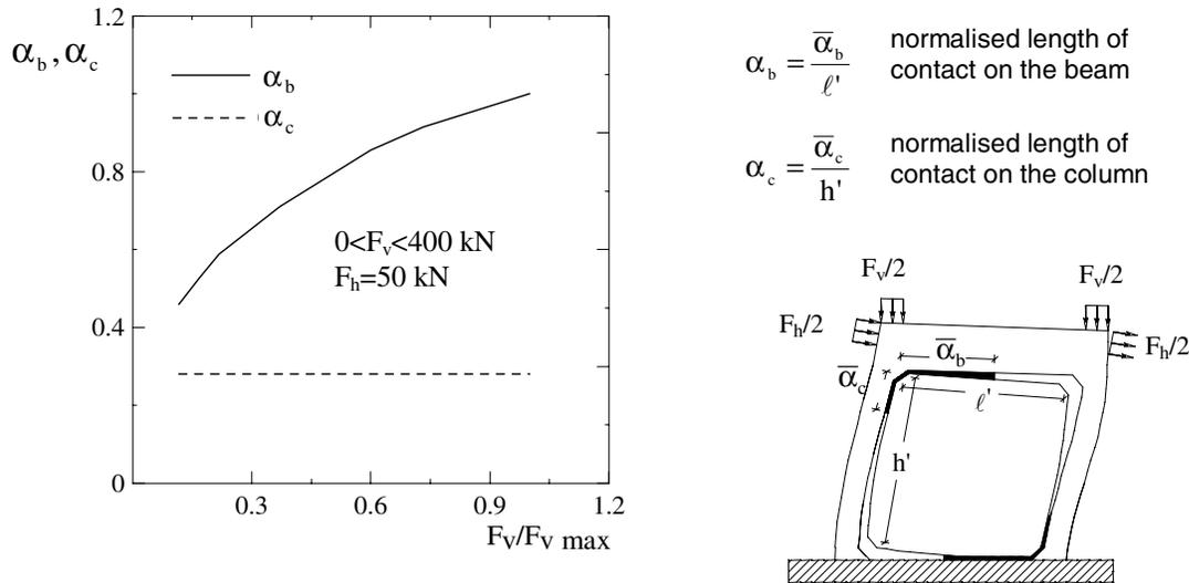
**Figure 5.** Lengths of contact ( $\alpha_b$ ,  $\alpha_c$ ) at the right upper corner
