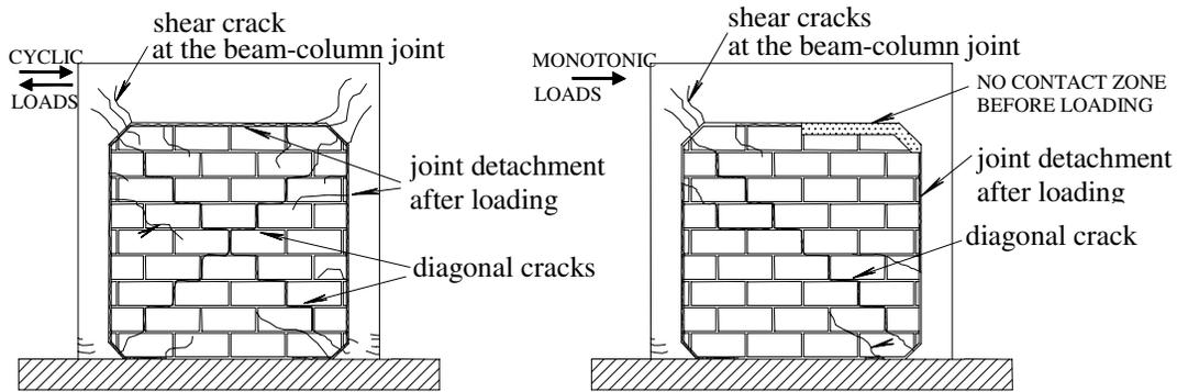
**Figure 9.** Crack distribution: a) infilled frame under cyclic lateral loads; b) infilled frame with partial frame-infill joint under monotonically increasing lateral loads.
