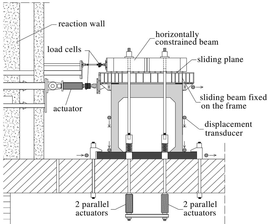
**Figure 8.** Test set-up
