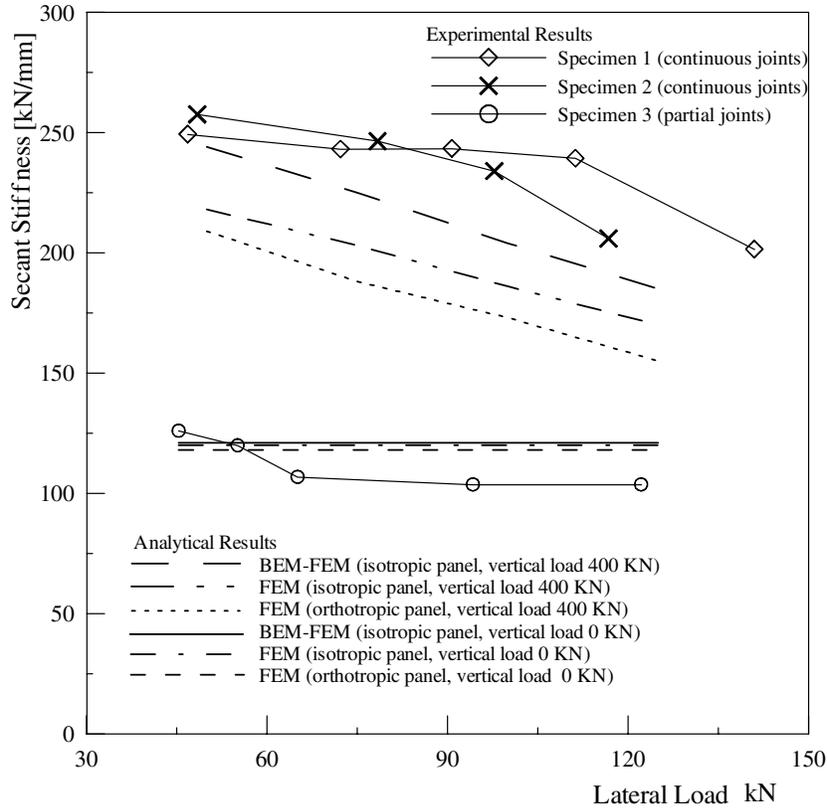
**Figure 12.** Comparison between experimental and analytical results.
