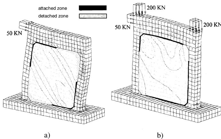
**Figure 10.** Flow of the stresses: a) reduced contact frame-infill; b) extended contact frame-infill
