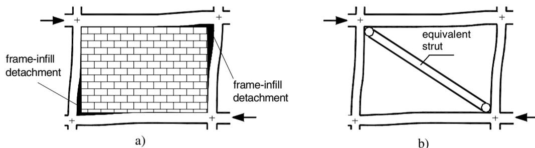
**Figure 3.** Infilled mesh: a) trend to detachment of frame from infill under lateral loads; b) strut equivalent to the infill
