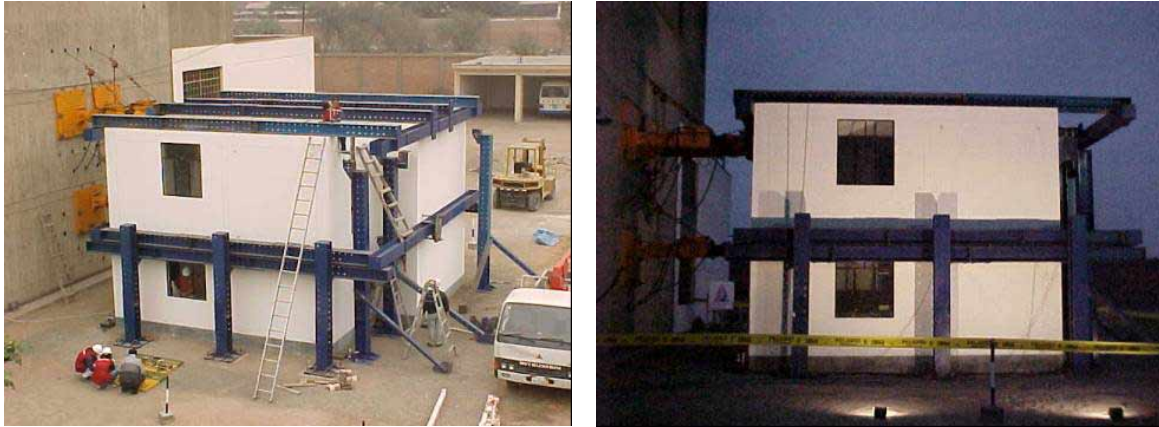
FIGURE 6: Test setup of the testing house
