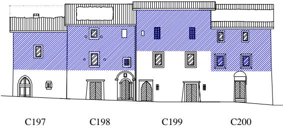
Fig. 10: Localization of the panels with lowest seismic coefficient (global overturning of a two floor wall) by simple kinematics models.
