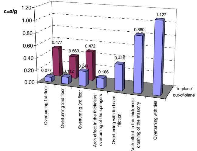
Figure 9: Comparison among the single kinematics models: the lowest seismic coefficients are related to the out-of-plane mechanisms involving the most damaged portions of the building.
