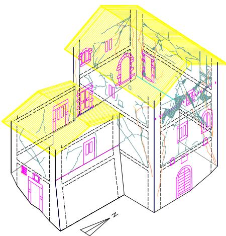
Figure 8: View of the building with survey of the crack pattern: the most damaged portions are the Eastern wall and the Nord-Eastern corner (overturning effects).
