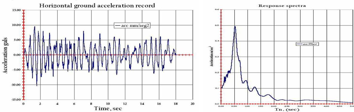
**Figure 11 – Horizontal ground acceleration recorded at Minatitlan, Veracruz**
