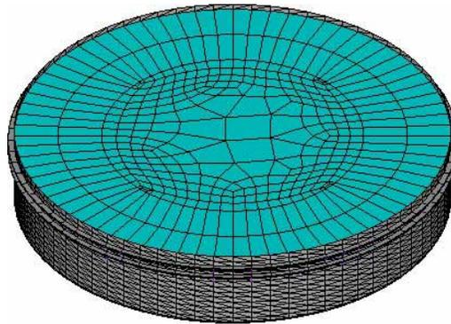
**Figure 5 - Model of cylindrical steel storage tanks of 500 thousands barrels**
