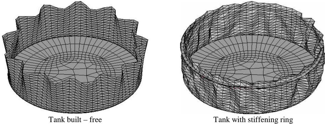
**Figure 7 – Mode shapes results of the empty tank of 200 thousands barrels,  $t=32.16$ mm**
