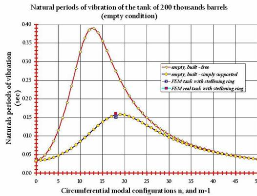
**Figure 6 - Natural periods of the tank of 200 thousands barrels (empty condition).**
