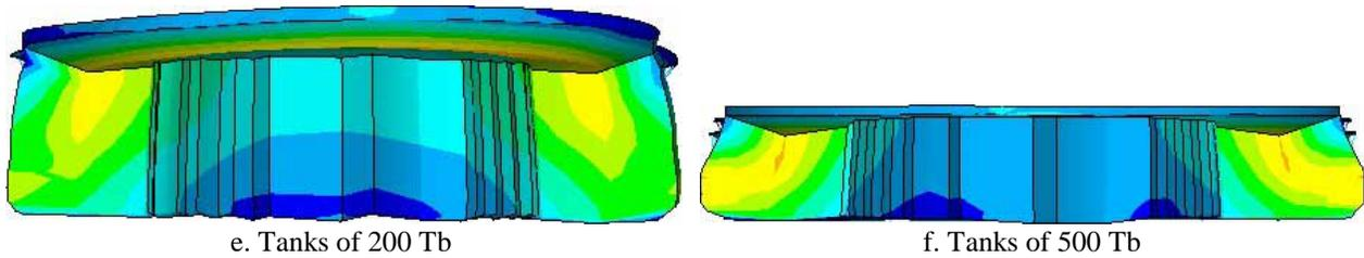
**Figure 17 – Configurations of seismic response of the two tanks studied**
