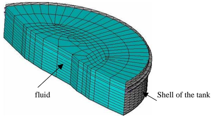
**Figure 9 – Model of analysis of the fluid – structure interaction system**
