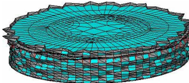
**Figure 10 – Modal shapes of the tank of the 500 Tb with a natural period of vibration.**
