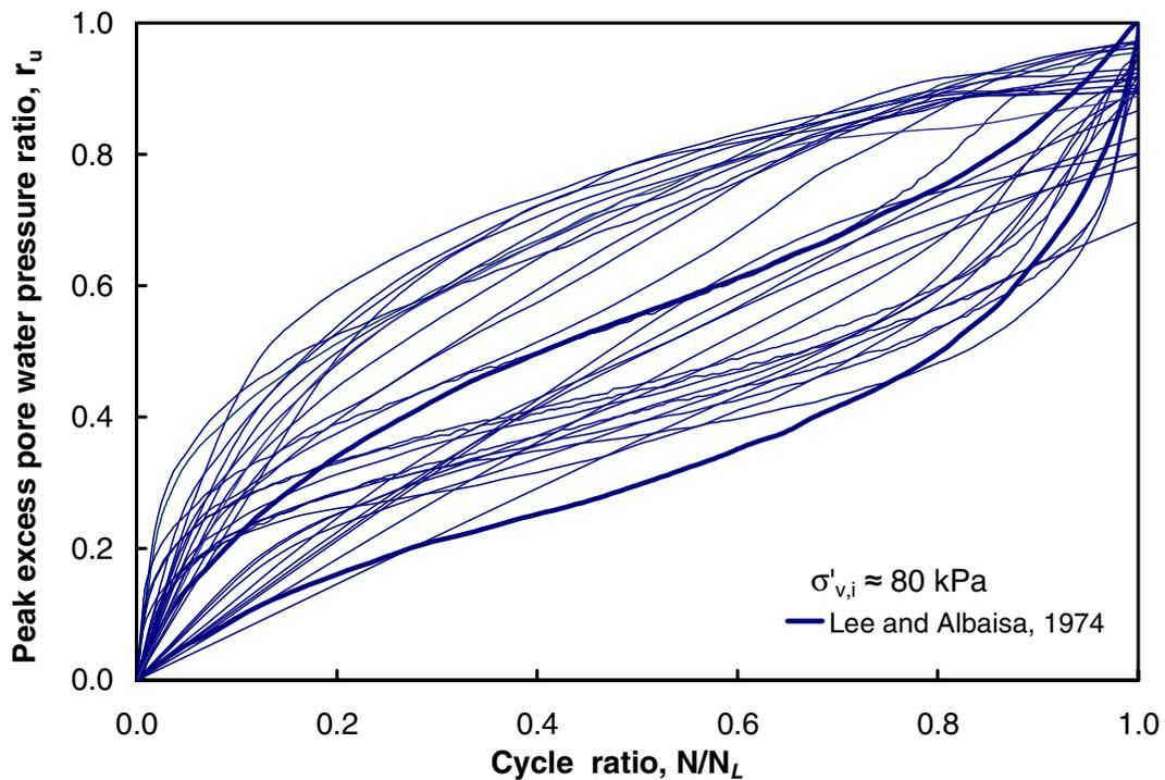
Figure 6: Pore water pressure buildup in cyclic simple shear tests
