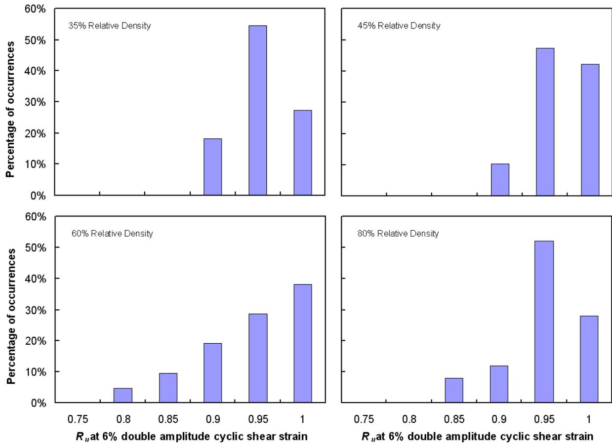
**Figure 8: Occurrence rates of pore water pressure ratio at liquefaction triggering**
