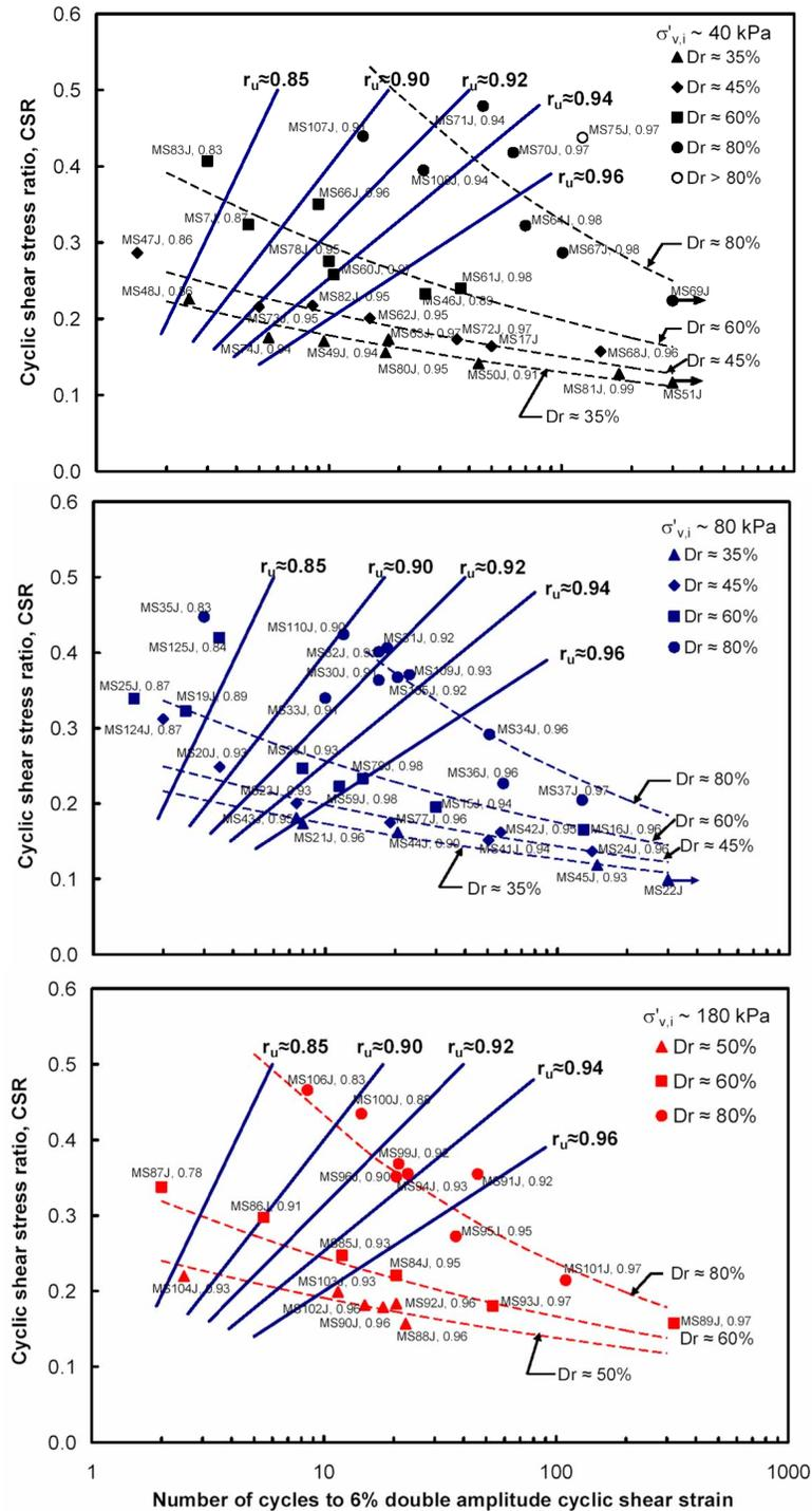
Figure 9: Relationships between pore water pressure ratio, relative density, and cyclic stress ratio
