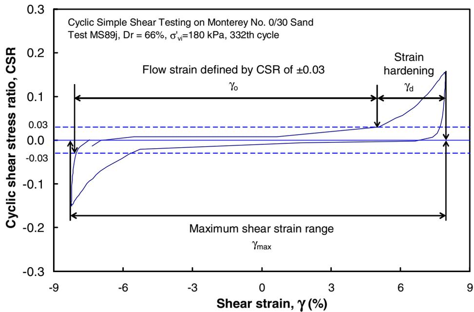
**Figure 3: Relationship between flow strain amplitude and maximum shear strain in this study**
