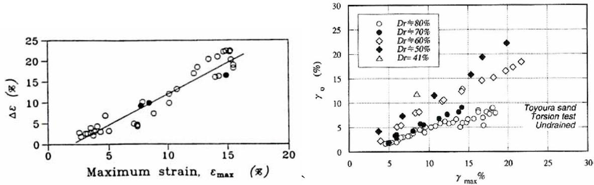
**Figure 4: Relationship between flow strain component and the preceding maximum cyclic strain in triaxial tests (left: Vaid and Tomas [8]), and in torsional tests (right: Shamoto et al. [9])**
