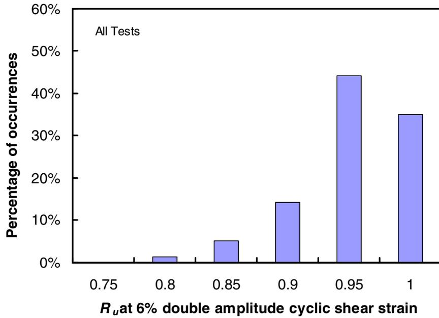
**Figure 7: Distribution of pore water pressure ratio at liquefaction triggering**
