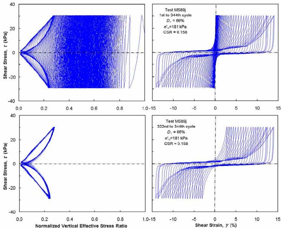
Figure 2: An example of post-liquefaction behavior of Monterey No. 0/30 sand
