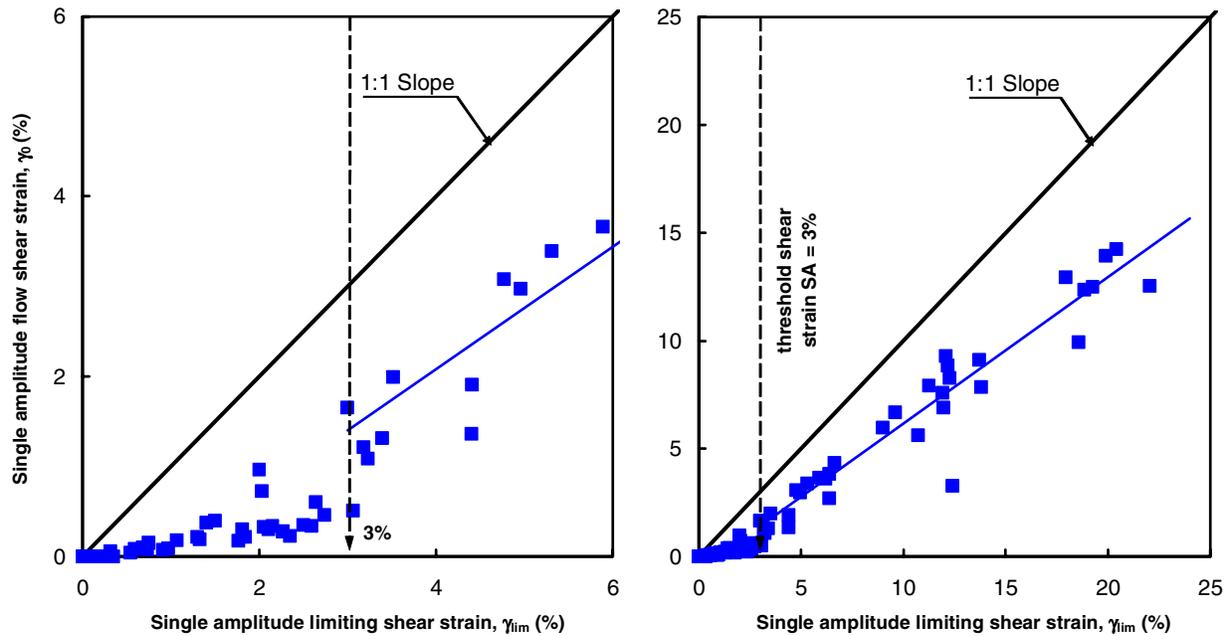
**Figure 5: Correlations between the flow strain and the limiting shear strain**
