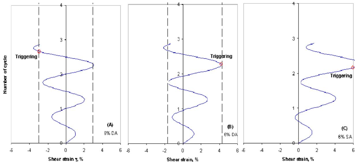
**Figure 1: Strain-based liquefaction triggering criteria in this study for (A) symmetrical cyclic loading and, (B) and (C) asymmetrical cyclic loading**
