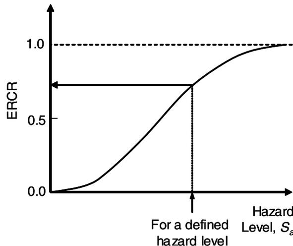
Figure 2 A typical hazard–loss relationship and its use.
