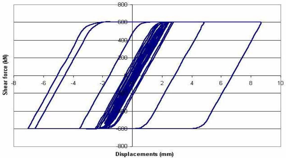
Figure 10. Hysteretic loop of a typical 600kN friction damper
