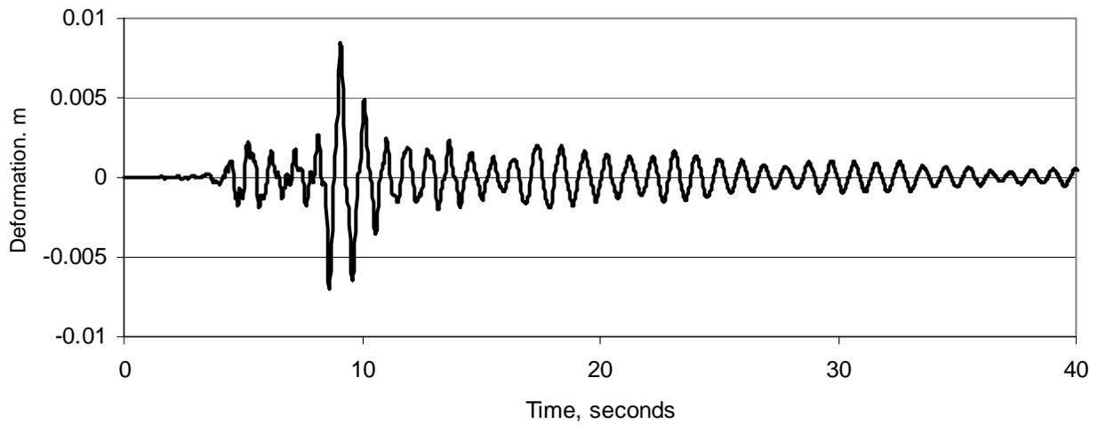
Figure 11. Time history of slippage of a typical 600kN friction damper
