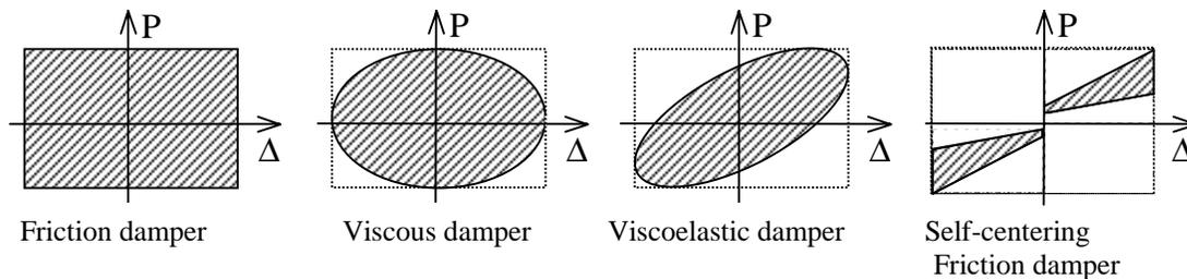
Figure 6. Comparison of hysteresis loops of different dampers
