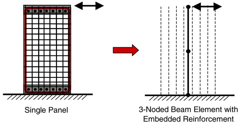
**Figure 7: Modeling the panels as fixed beams.**
