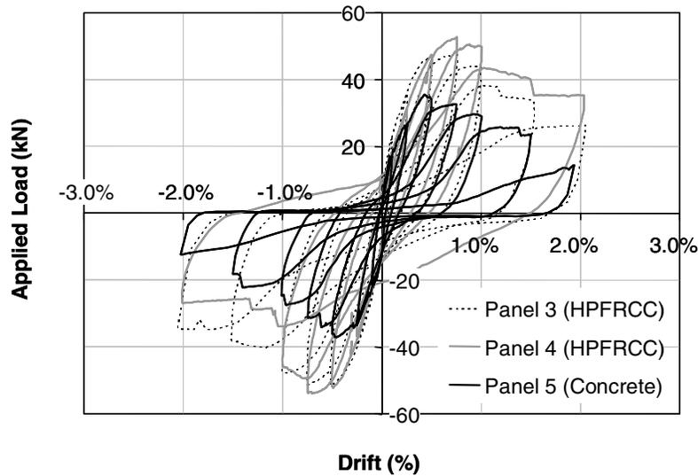
**Figure 6: Hysteretic response of single panels under cyclic lateral loading up to 2% drift.**
