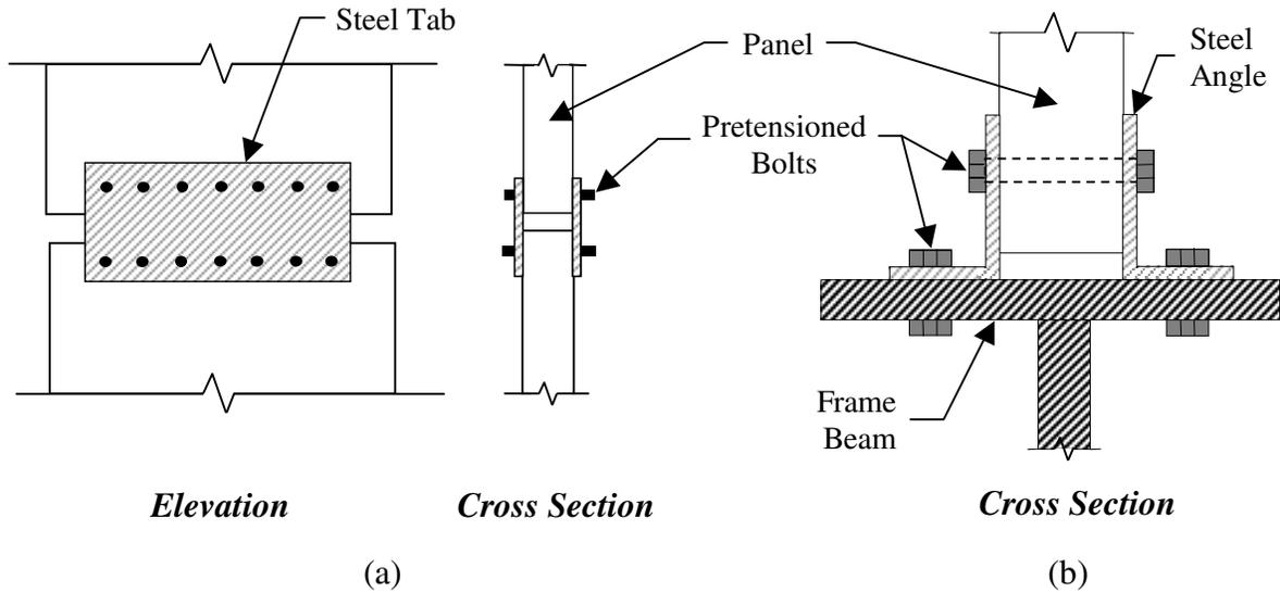
**Figure 2: Connection details for panel-to-panel connections (a) and panel-to-frame connections (b).**
