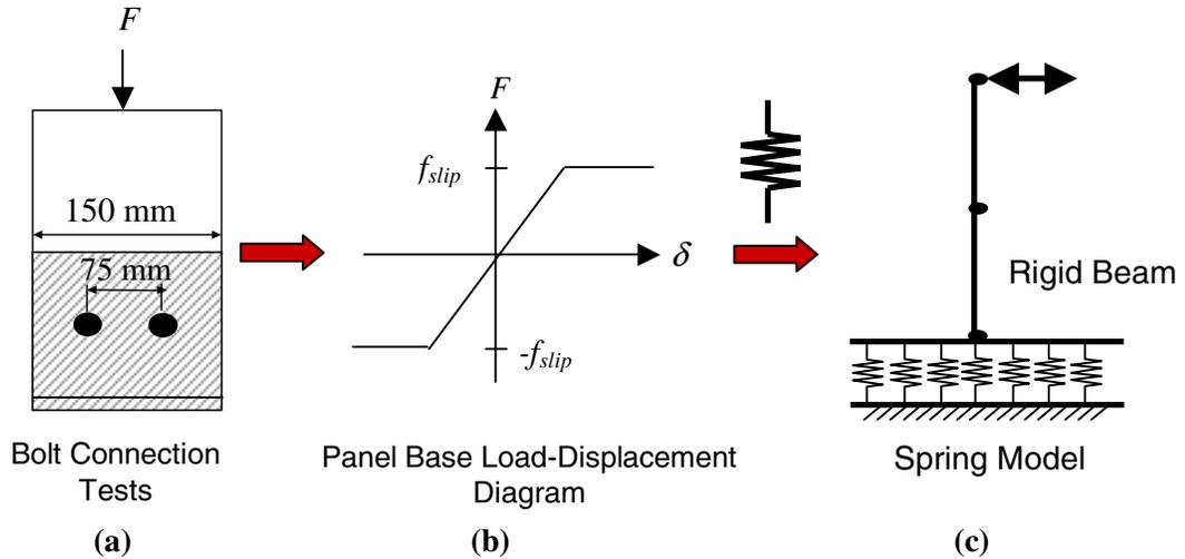
**Figure 11: Development of a connection-slip model for the panels.**
