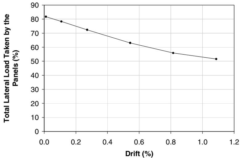
**Figure 15: Proportion of lateral load carried by the panels for the beam element frame model.**
