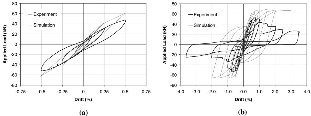
**Figure 10: Hysteretic behavior for the fixed beam panel model in the initial cycles (a) and full response (b)**
