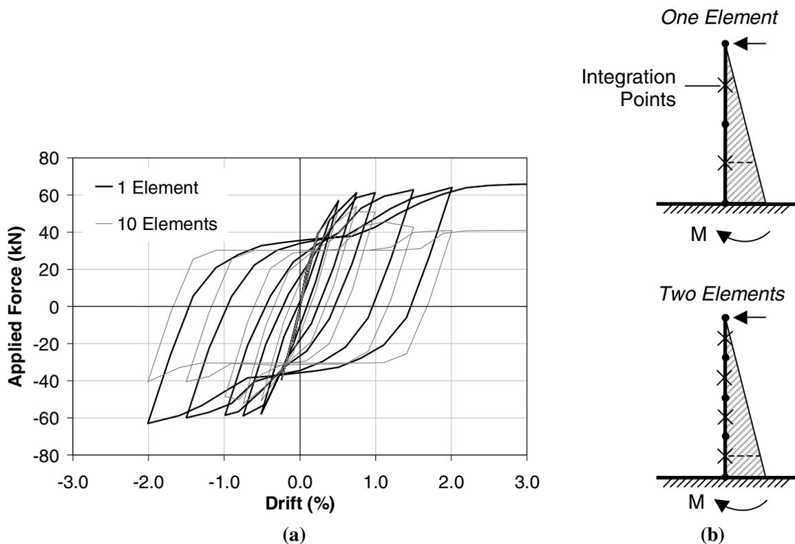
**Figure 9: Mesh sensitivity in the panel model (a) resulting from increased element stresses (b).**
