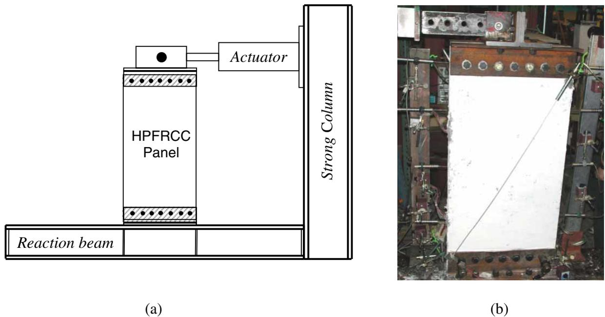
**Figure 5: Test set-up for cyclic lateral load experiments on single panels (a), and a panel specimen just prior to testing (b).**
