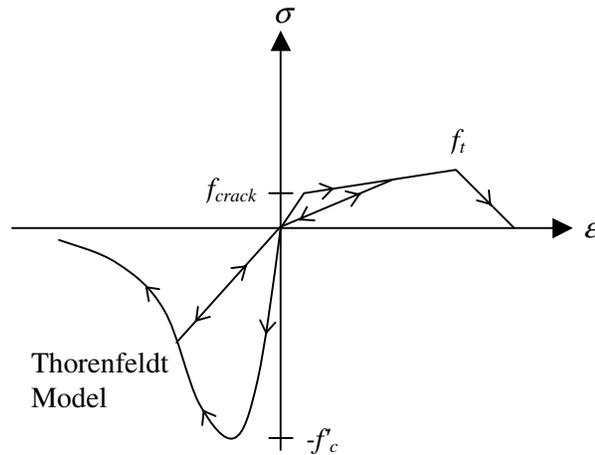
**Figure 8: Idealized stress-strain relationship for the HPFRCC.**
