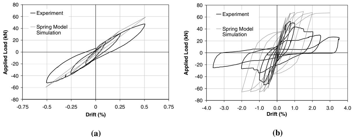
**Figure 12: Hysteretic response of the panel when slip in the connection region is modeled: initial cycles (a) and full response (b).**
