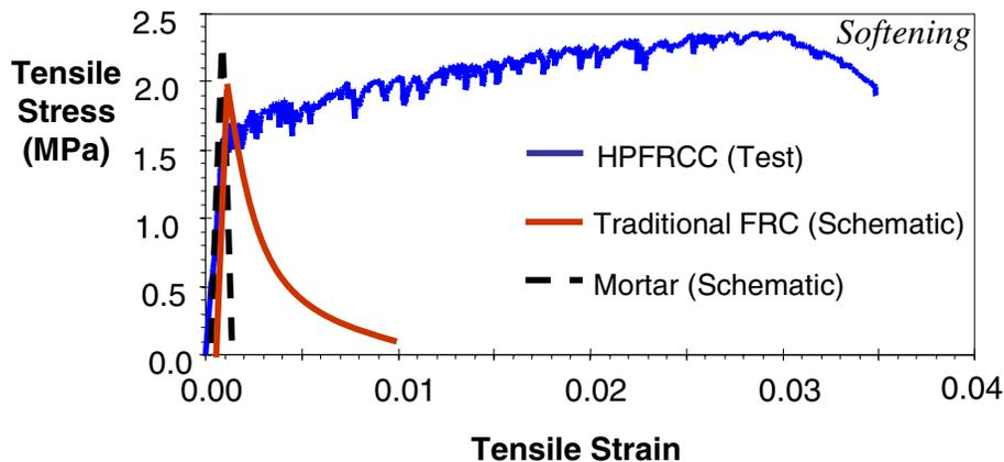
Figure 4: Uniaxial tensile response of HPFRCC materials.
