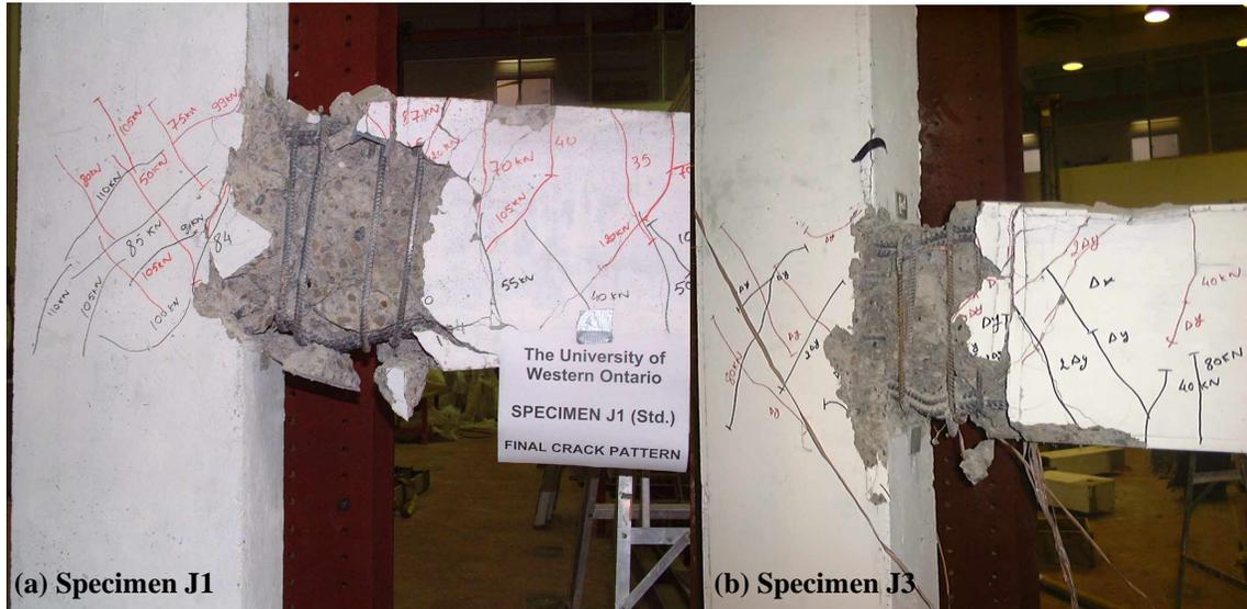
Figure 6. Final crack pattern for (a) NC specimen (*J1*), and (b) SCC specimen (*J3*).
