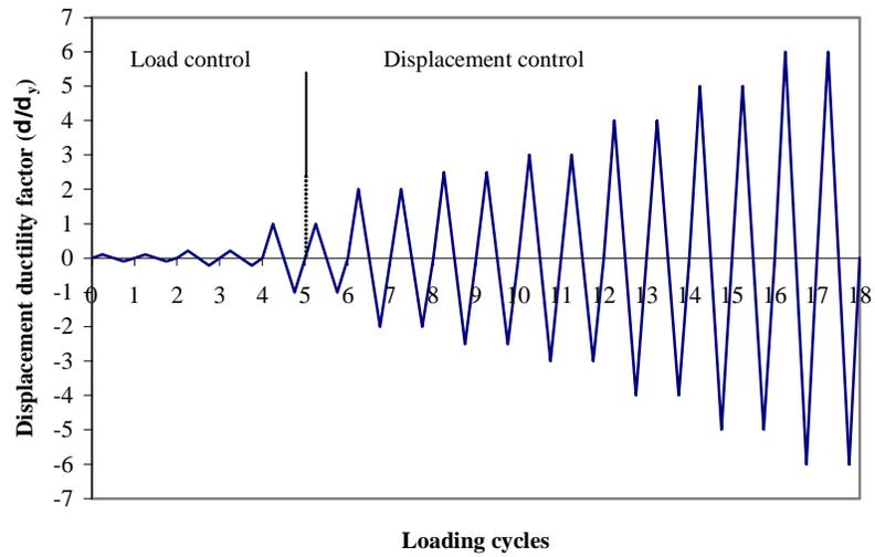
Figure 2. Load history for the reversed cyclic load test used in this study.
