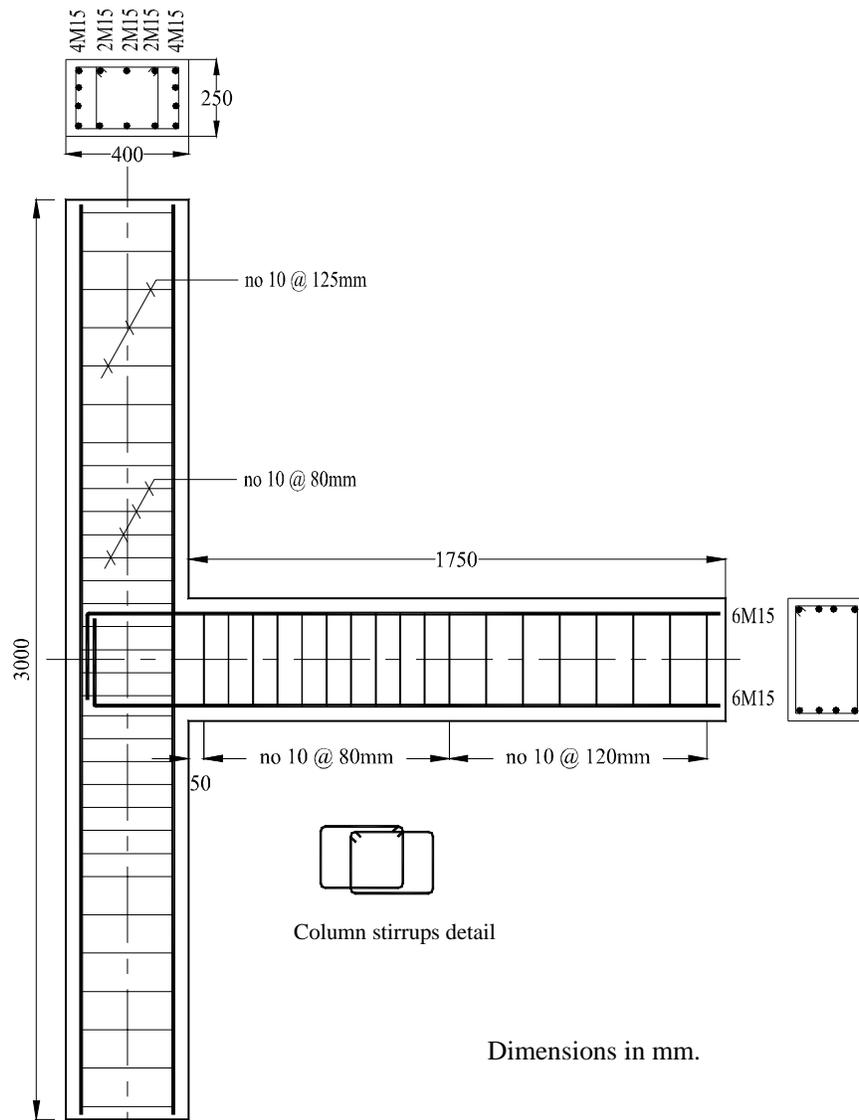
**Figure 1. Reinforcement details for the specimens.**
