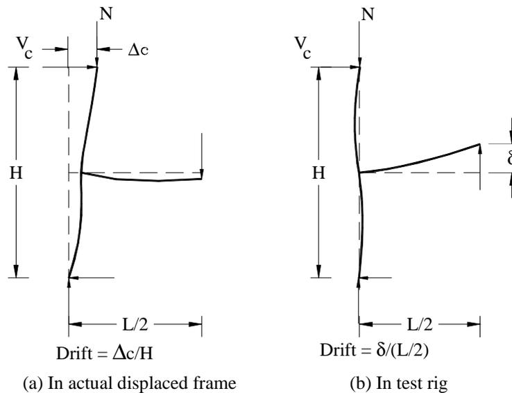
**Figure 10. Exterior beam-column subassemblages in (a) displaced frame and (b) test rig.**
