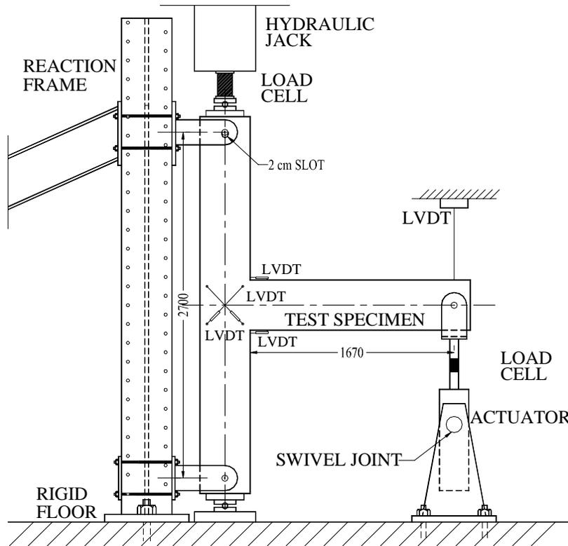
Figure 3. Test setup.
