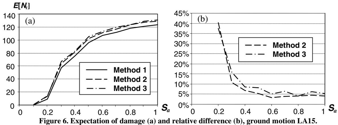
Figure 6. Expectation of damage (a) and relative difference (b), ground motion LA15.
