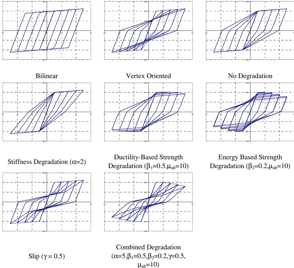
**Figure 3. Capabilities of the polygonal hysteretic model**
