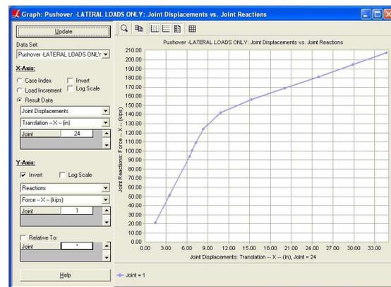
Figure 25. Base shear-root displacement plot
