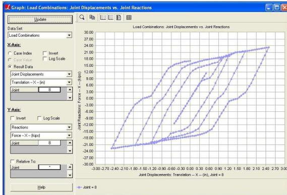
Figure 13. Force-displacement plot in the x-direction
