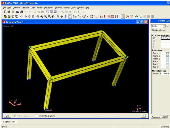
Figure 11. 3D Frame model
