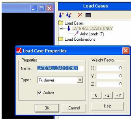
Figure 22. Pushover load-case configuration
