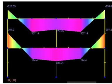
Figure 28. Moment diagram after member removal
