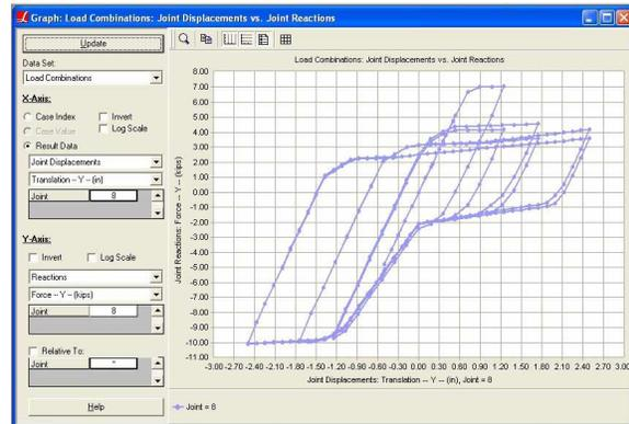
Figure 14. Force-displacement plot in the y-direction
