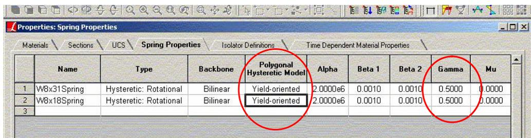
Figure 10. Hysteretic parameters for slip behavior
