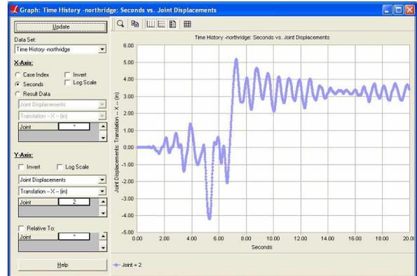
**Figure 30. Nonlinear time-history analysis of a portal frame subject to Northridge earthquake (Displacement time-history of top node)**
