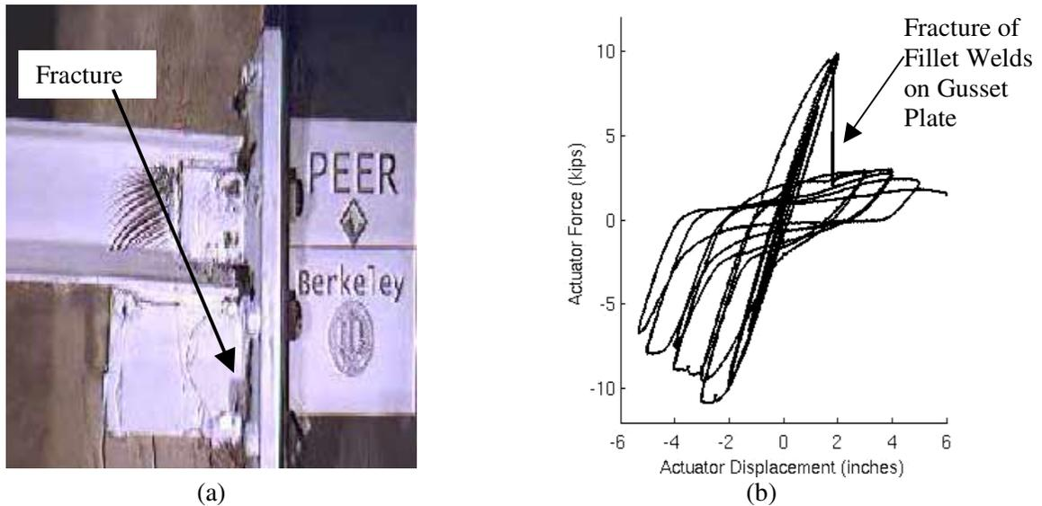
**Figure 9. Simple Beam to Column Connection, (a) Photo and (b) Hysteresis**
