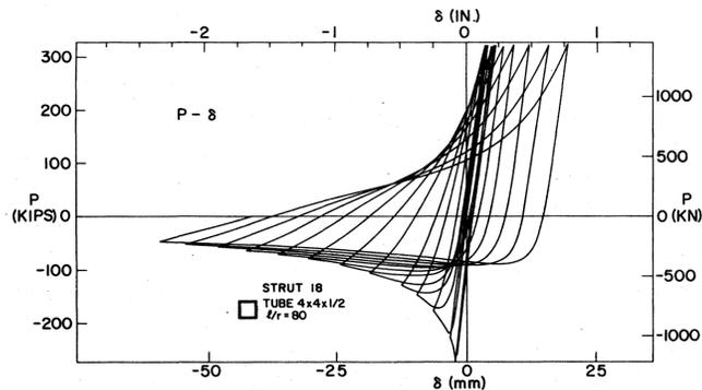
Figure 3. Experimental Test Results of Tubular Strut
