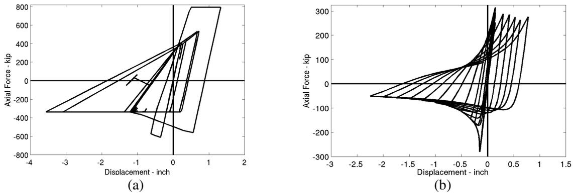
Figure 4. (a) Phenomenological Numerical Hysteresis (SNAP-2DX). (b) Tubular Strut Modeling in OpenSees
