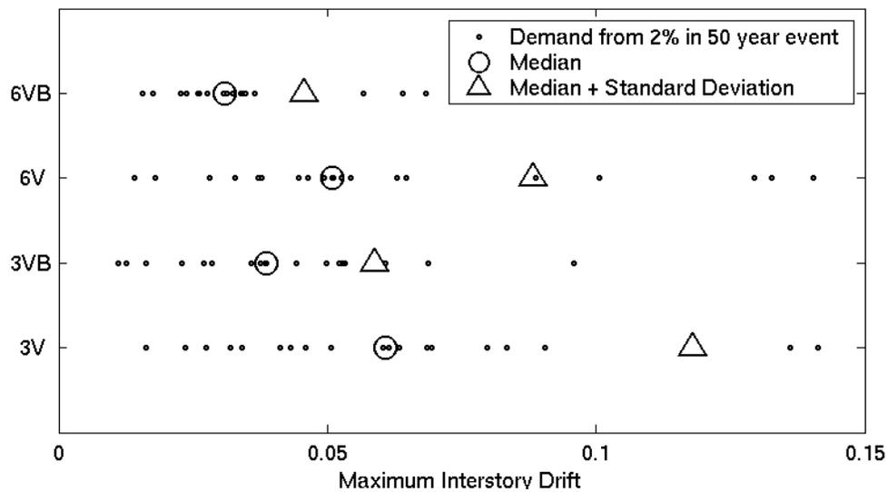
**Figure 2. 2% in 50 Year Drift Demands for 3V, 3VB, 6V and 6VB Structure.**
