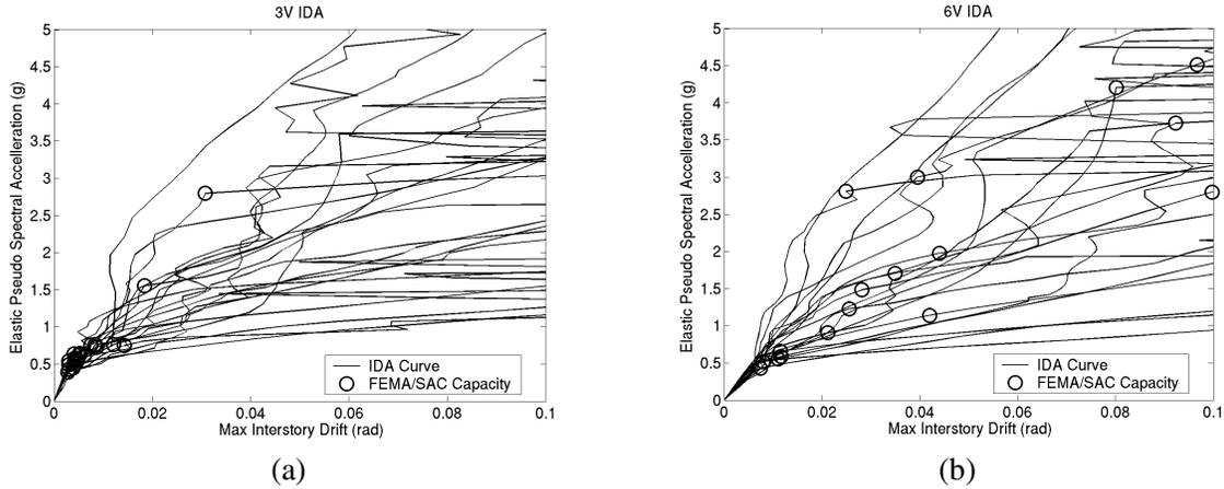
**Figure 5. Incremental Dynamic Analysis for (a) 3V and (b) 6V**
