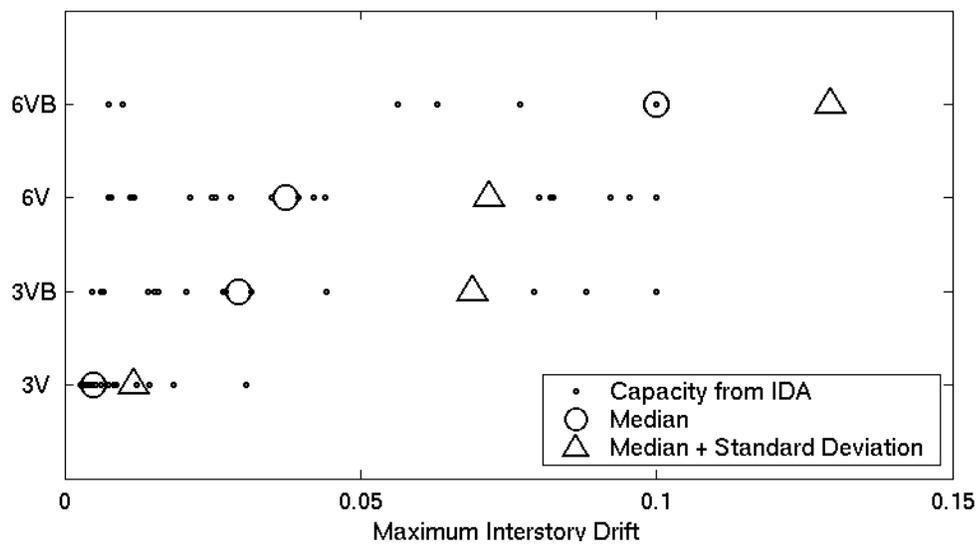
**Figure 7. Incremental Dynamic Analysis Capacity Results for special concentric and buckling restrained braced frames**
