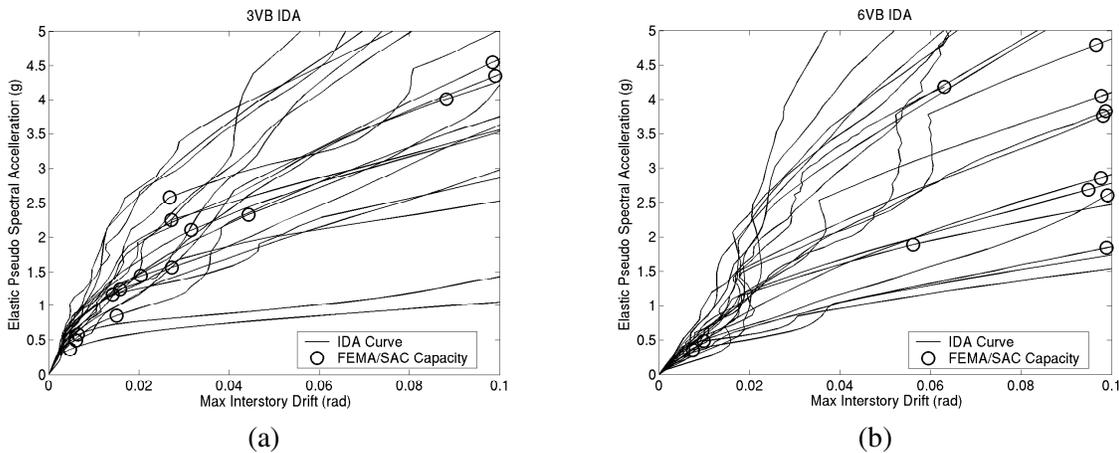
**Figure 6. Incremental Dynamic Analysis for (a) 3VB and (b) 6VB**
