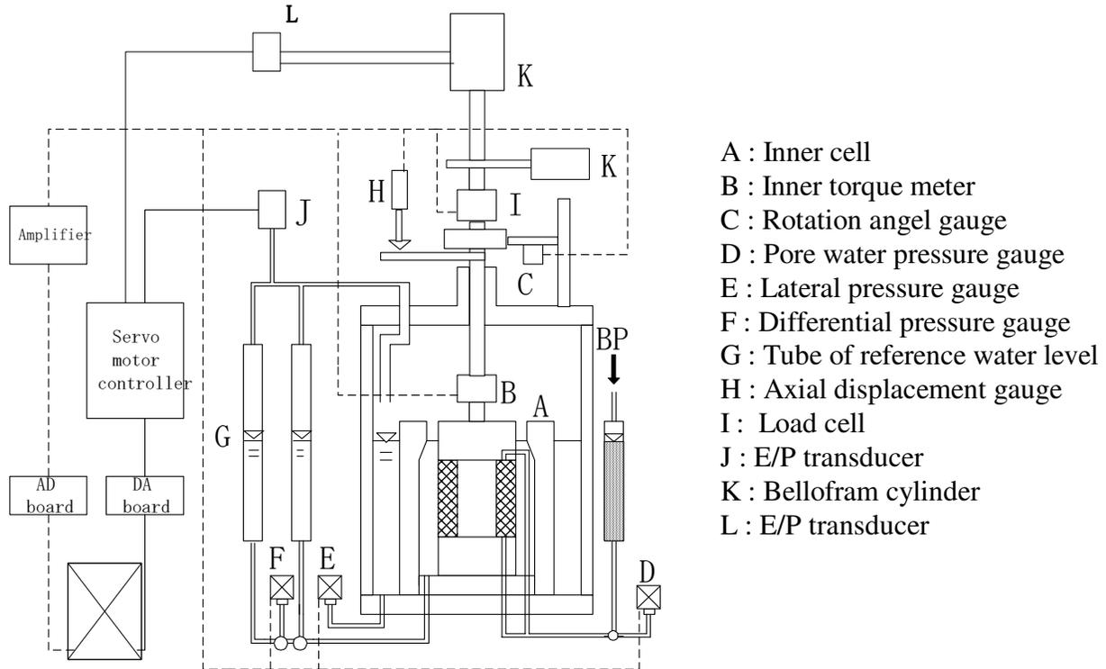
**Fig.1 The schematic illustration of the cyclic torsional shear apparatus**
