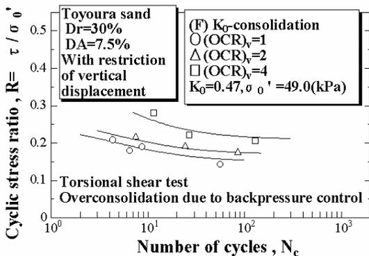
Fig. 13 Cyclic stress ratio,  $R$ , versus number of cycles,  $N_c$ , to  $DA=7.5\%$
