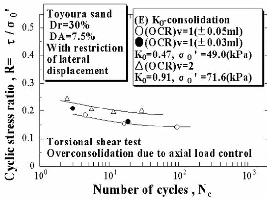
Fig. 11 Cyclic stress ratio,  $R$ , versus number of cycles,  $N_c$ , to  $DA=7.5\%$
