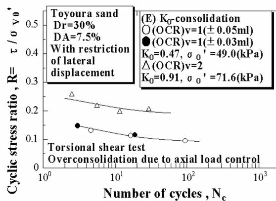
Fig. 12 Cyclic stress ratio,  $R$ , versus number of cycles,  $N_c$ , to  $DA=7.5\%$
