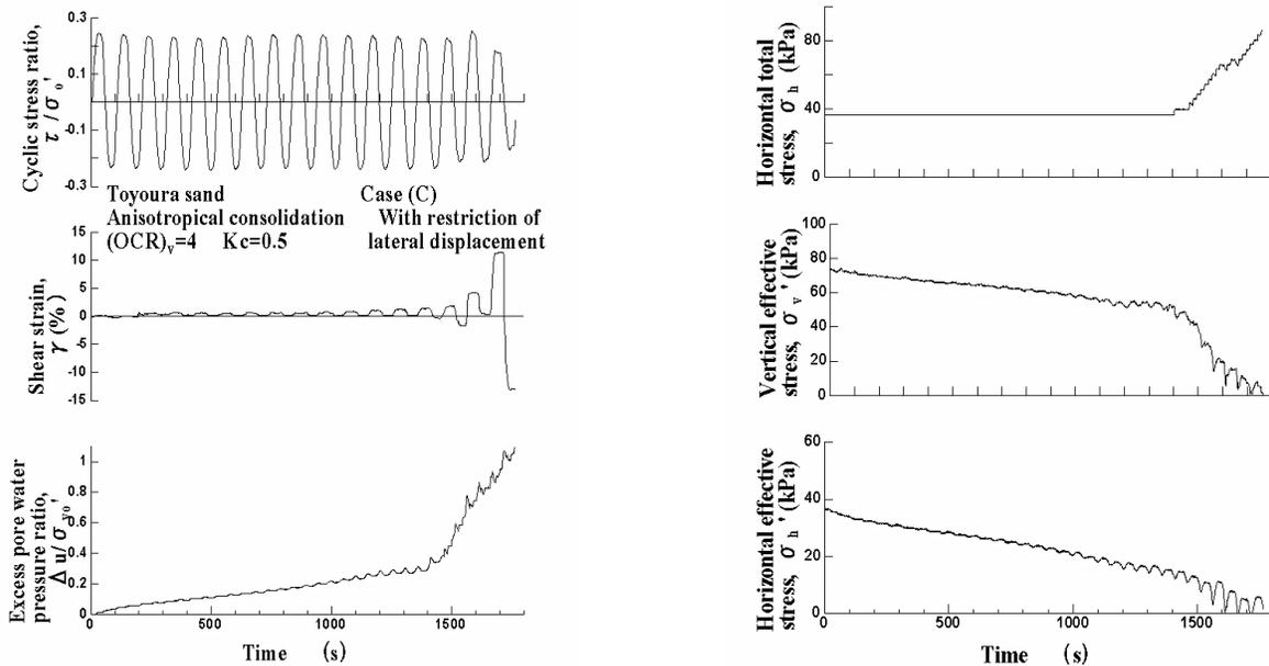
**Fig.5 Typical time histories of test results observed in Case(C)**
