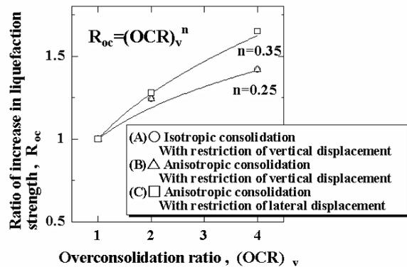
**Fig. 8 Ratio of increase in liquefaction strength,  $R_{oc}$ , versus overconsolidation ratio,  $(OCR)_v$**
