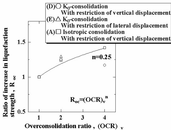
**Fig. 15** Ratio of increase in liquefaction strength,  $R_{oc}$ , versus overconsolidation ratio,  $(OCR)_v$
