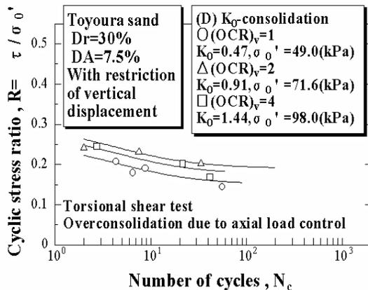
**Fig. 9 Cyclic stress ratio,  $R$ , versus number of cycles,  $N_c$ , to  $DA=7.5\%$**
