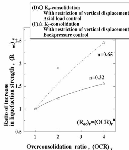
**Fig. 18** Ratio of increase in liquefaction strength,  $(R_{oc})_v$ , versus overconsolidation ratio,  $(OCR)_v$
