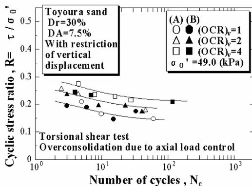
Fig. 6 Cyclic stress ratio,  $R$ , versus number of cycles,  $N_c$ , to DA=7.5%
