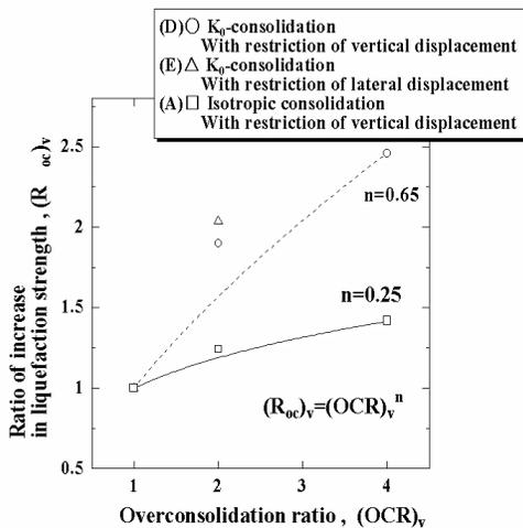
**Fig. 17** Ratio of increase in liquefaction strength,  $(R_{oc})_v$ , versus overconsolidation ratio,  $(OCR)_v$
