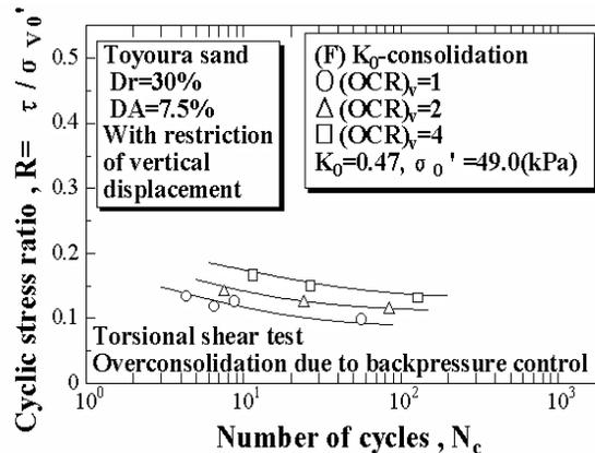
Fig. 14 Cyclic stress ratio,  $R$ , versus number of cycles,  $N_c$ , to  $DA=7.5\%$
