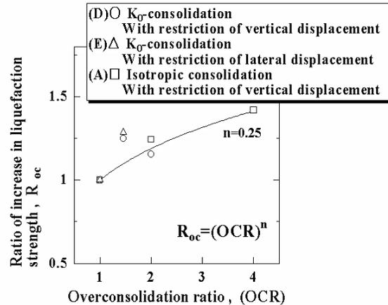
**Fig. 16** Ratio of increase in liquefaction strength,  $R_{oc}$ , versus overconsolidation ratio,  $(OCR)_v$
