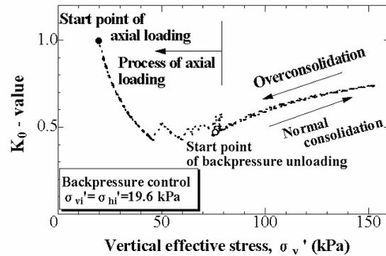
**Fig.3** Coefficient of earth pressure at rest, K<sub>0</sub>, versus vertical effective stress,  $\sigma_v'$
