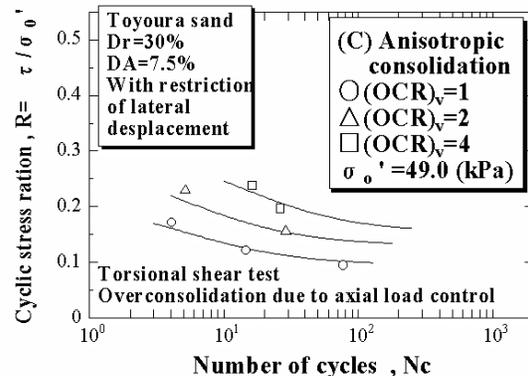
Fig. 7 Cyclic stress ratio,  $R$ , versus number of cycles,  $N_c$ , to DA=7.5%
