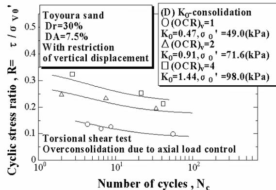
**Fig. 10 Cyclic stress ratio,  $R$ , versus number of cycles,  $N_c$ , to  $DA=7.5\%$**
