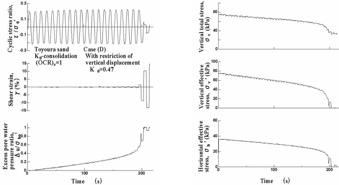
**Fig.4 Typical time histories of test results observed in Case(D)**
