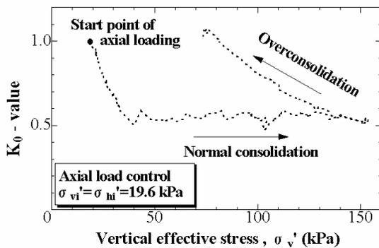
**Fig.2** Coefficient of earth pressure at rest, K<sub>0</sub>, versus vertical effective stress,  $\sigma_v'$
