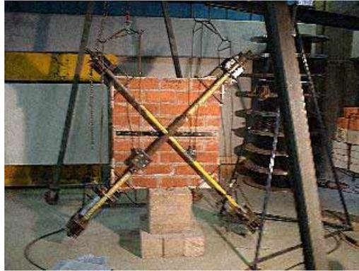
**Figure 2 Test setup for cyclic loading tests**
