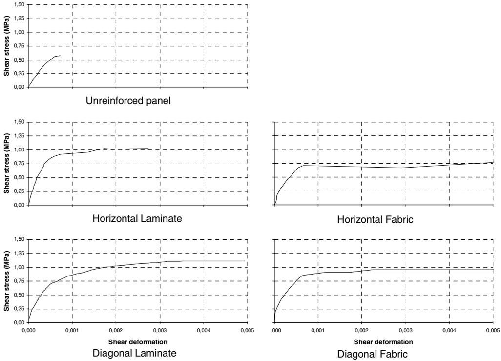
**Figure 3 Shear tension-shear deformation responses of masonry panels under monotonic loading**
