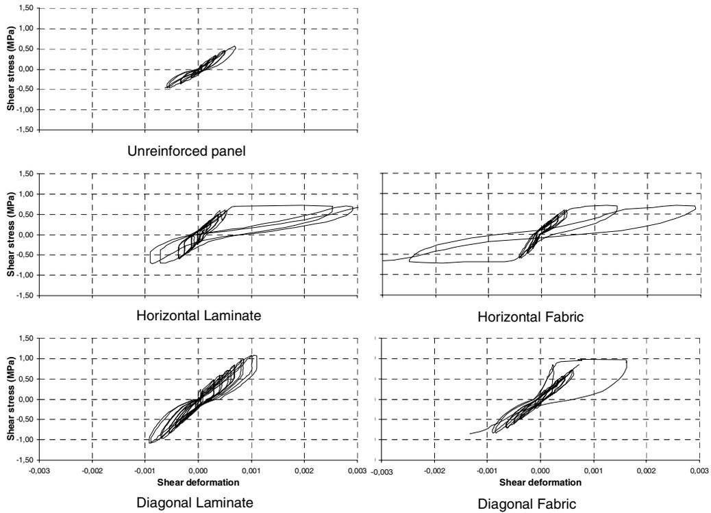
**Figure 4 Shear tension-shear deformation responses of masonry panels under cyclic loading**
