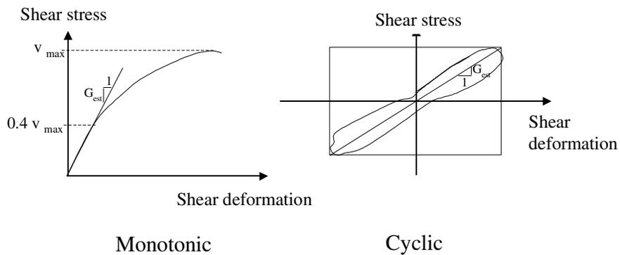
**Figure 6 Methods of calculation of the monotonic and cyclic shear modulus**
