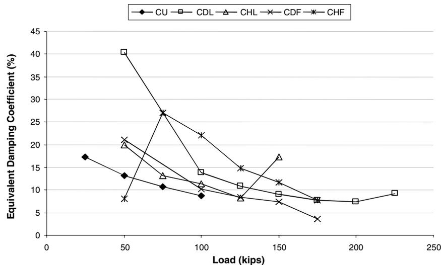
**Figure 8 Equivalent damping coefficient at various load levels**
