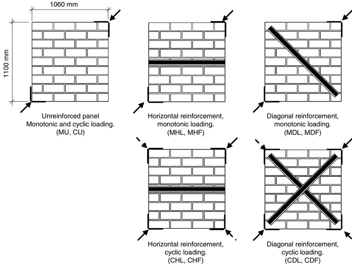
**Figure 1 Dimensions of the panels and configurations of the reinforcement**
