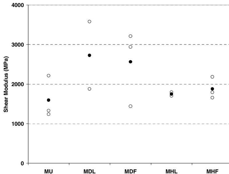
**Figure 7 Shear modulus of each specimen and average value for each reinforcement configuration**
