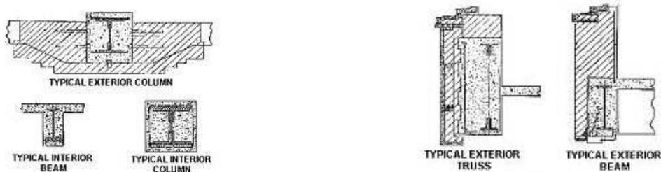
Figure 5. Typical beam and column sections
