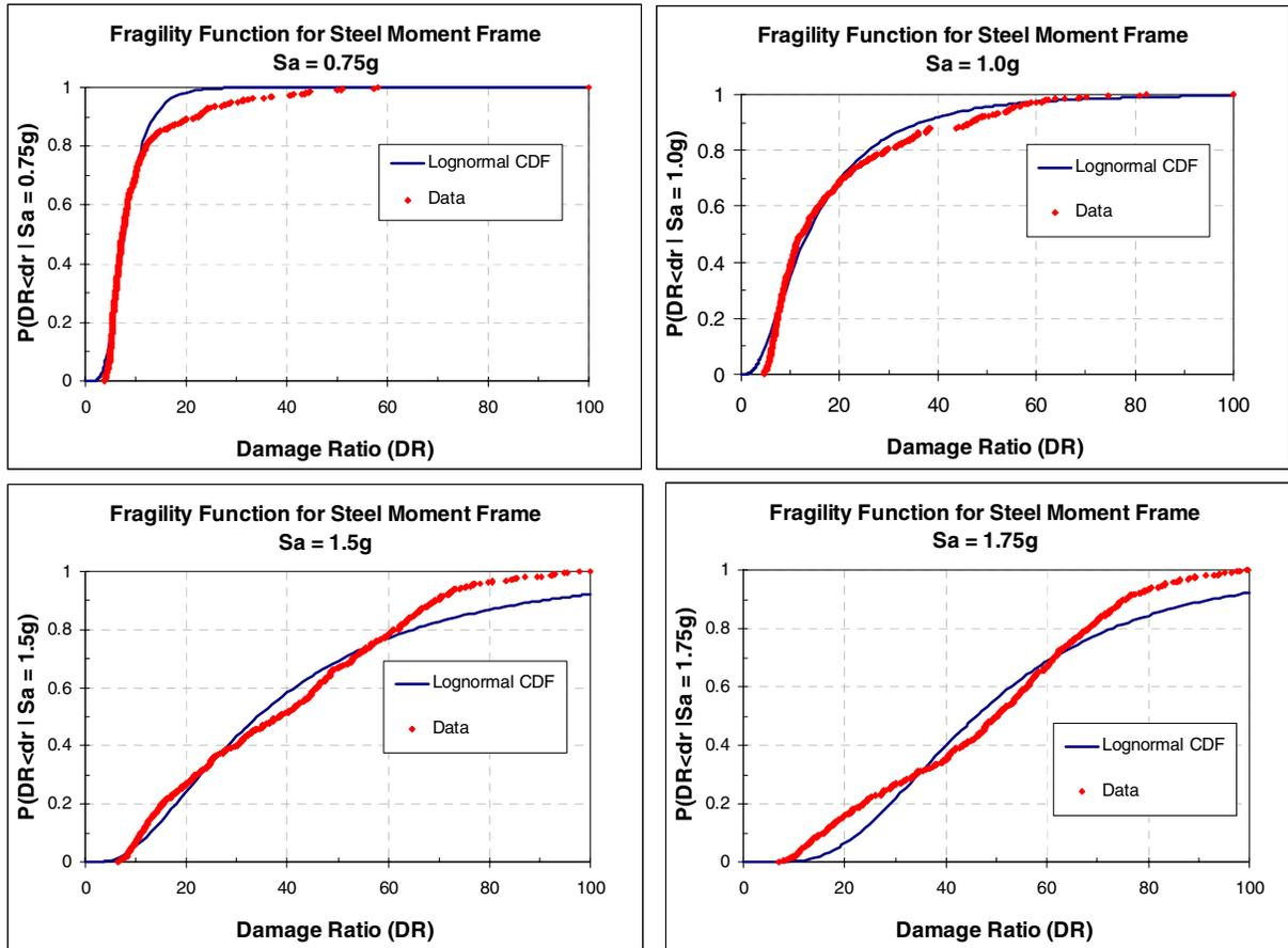
**Figure 3. Fragility functions for the 9-story SAC building for different spectral acceleration levels**
