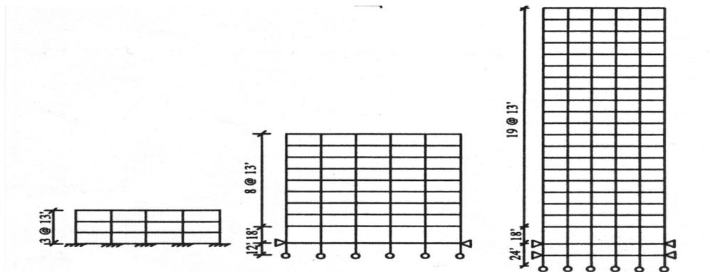
**Figure 2. Elevation views of the Three SAC Steel Moment Resisting Frames used in the Nonlinear Dynamic Analyses (Gupta and Krawinkler, 1999)**
