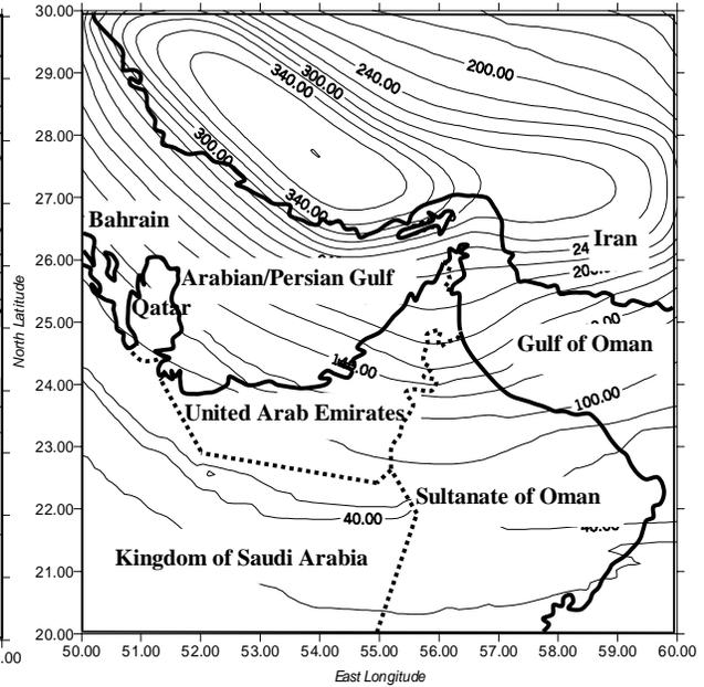
Figure 5. PGA ( $\text{cm} / \text{sec}^2$ ) for 100 years time
