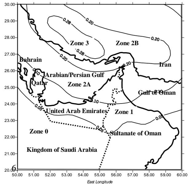
Figure 7. Seismic zoning map of UAE and its vicinity for 475 years return period showing five zones (0,1, 2A, 2B and 3)
