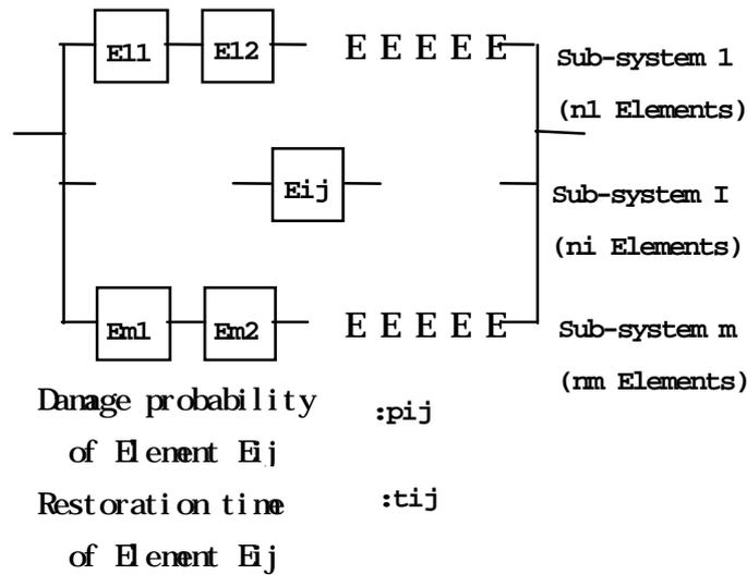
Figure 2 Illustration of serial-parallel system
