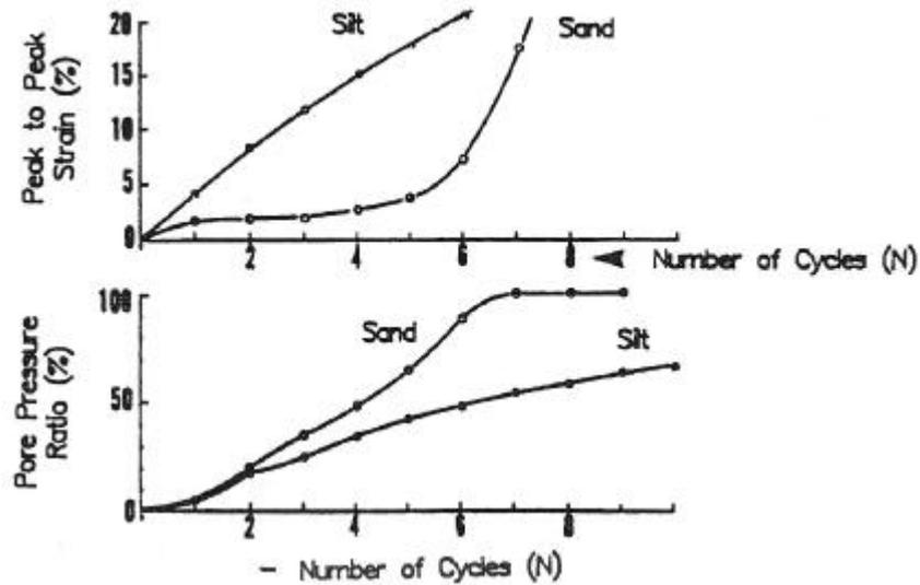
Figure 1. Comparison of Strain and Pore Pressure development in a typical Silt sample (after Singh, 1996)
